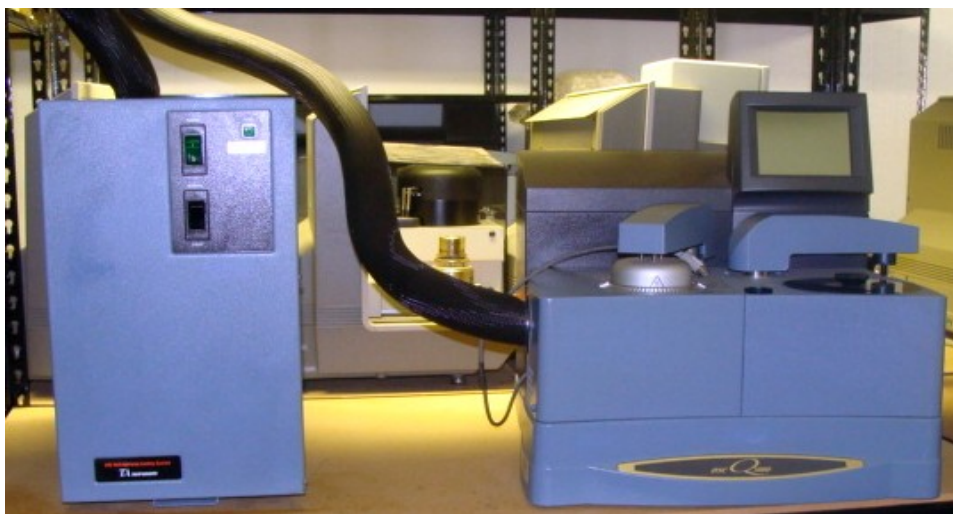
Fig. 4.3: Experimental setup of DSC Q100
