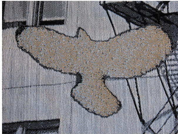
Fig. 4.29 Sensing bird from the Tapestry, woven with conductive thread.
