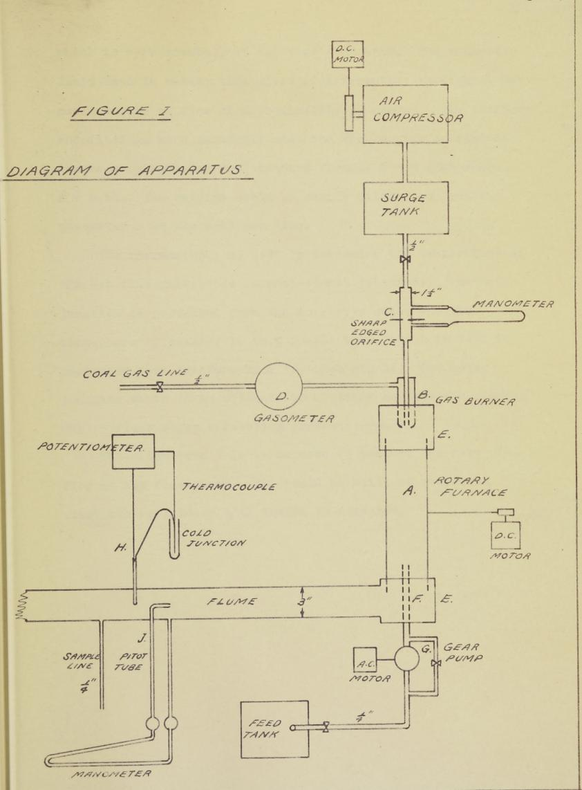
which is approximately at the vena contracta. The manometer fluid used is water; this gives a differential reading at the maximum rate of flow of approximately 20 cent. The orifice and fittings were carefully made and should give sufficient accuracy by applying the standard formula U = C VZgh where C = 0.61. The orifice could be easily calibrated from the gasometer D on the coal gas line.
