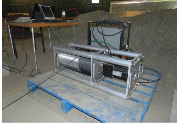
FIGURE 4.14. A winch was used to control the translational velocity of the rover
