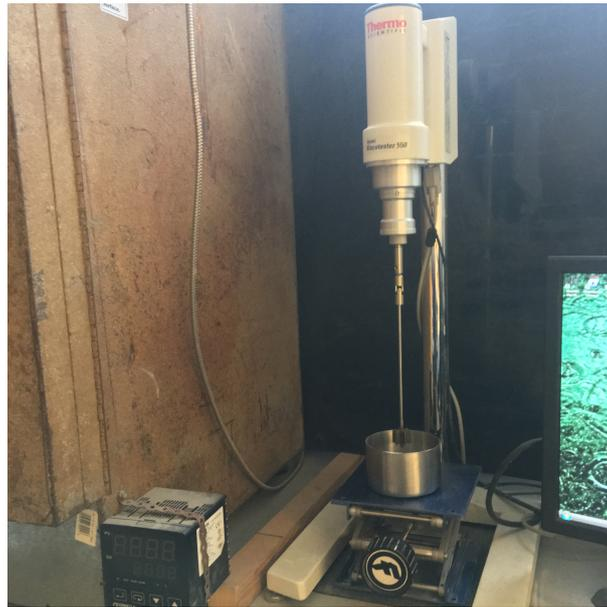
**Figure 3.13:** Vane attachment in the rheometer for yield stress measurement
