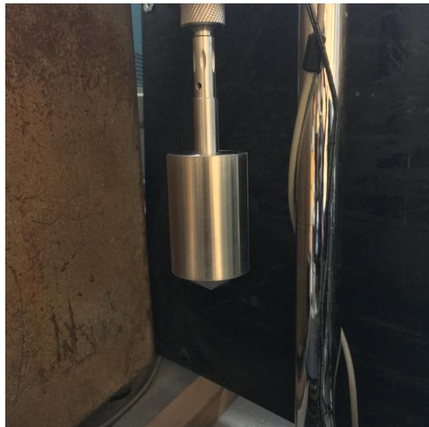
**Figure 3.5:** Bob attachment in the viscometer for yield stress and consistency index measurement
