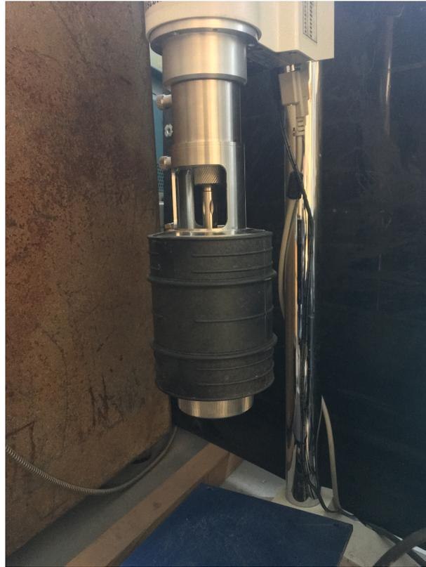
**Figure 3.6:** Cup and bob attachment with outer jacket for water circulation
