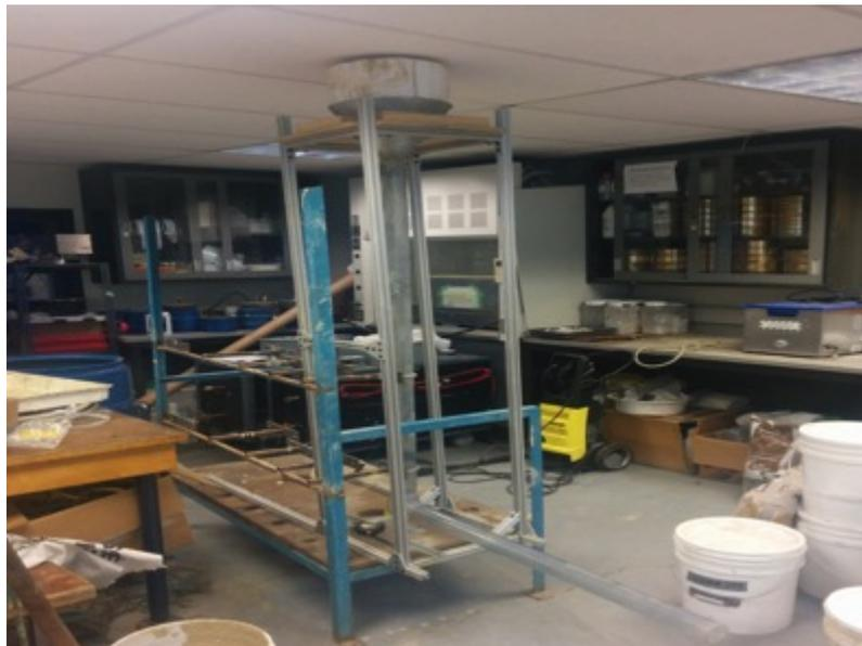
**Figure 5.1:** L-pipe arrangement used in the laboratory
