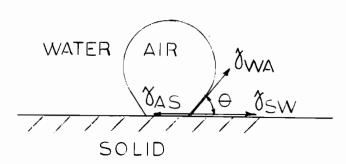
If %as, %sw and %aw are the surface tensions in dynes/cm, equivalent to surface energies at the interfaces of air solid, solid water and water air respectively, it may be shown thermodynamically that a necessary condition for a bubble adhesion is that there will be a reduction in the surface free energies as adhesion takes place.
