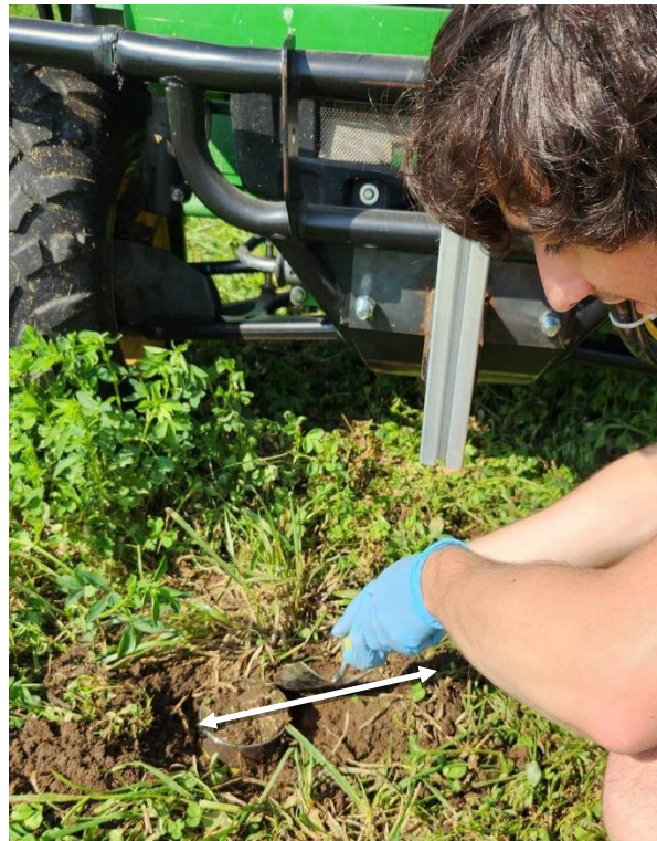
Figure 3.20: Core sampling process showing the distance from probe sampling location
