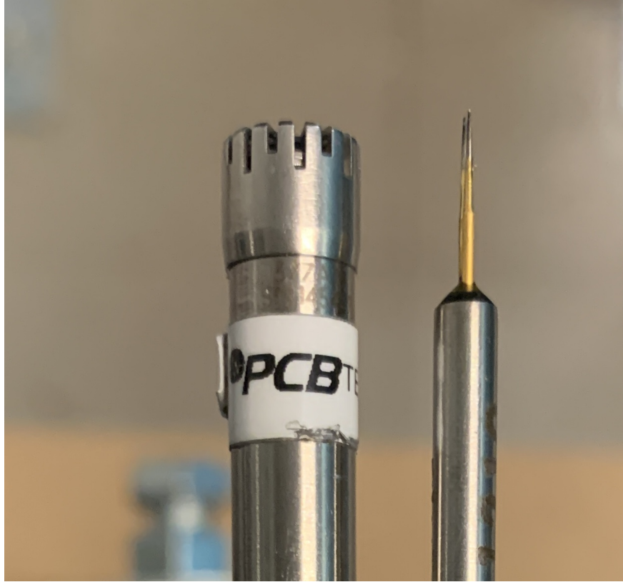
Figure 17: Combination of a condenser microphone with a hot-wire probe.
