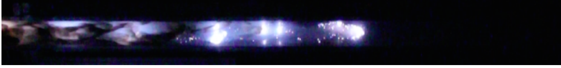
Figure 2–5: Picture of magnesium flame propagating upwards in a vertical tube. Image has been rotated so flame is propagating from the left to the right. Large sections of the tube can be seen burning simultaneously, beneath the flame front.
