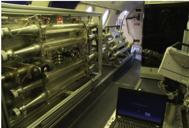
(a) Microgravity apparatus installed onboard Falcon-20 aircraft.
