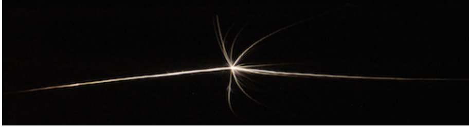
Figure 4-5: Long exposure photograph from DSLR of iron particle with impurities terminating with explosion during burning process.
