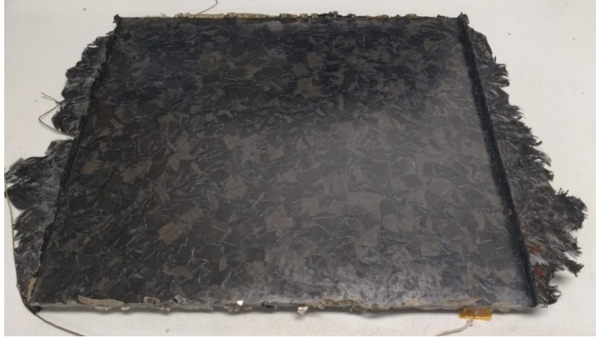
Figure 31: Moulded 304.8 mm x 355.6 mm panel, made with square strands, showing excessive material leakage (flashing) along 304.8 mm sides of the panel.
