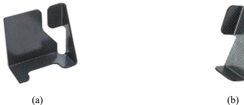
Figure 1: Thermoformed thermoplastic (a) “Auto-Stabilized” clip and (b) “Cleat” used to attach the composite fuselage of the Airbus A350 to its frame [8].
