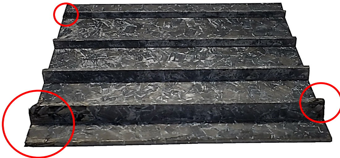
Figure 63: Insufficient fill seen in Rib A and Rib D when moulded with short strands at 10 bar filling pressure and 400°C at the temperature controller. Areas of insufficient fill circled in red.
