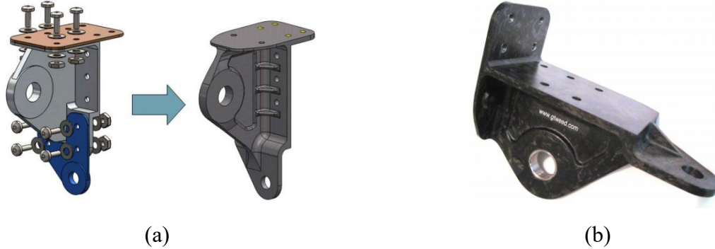
Figure 4: Industry example of DLF part replacing assembly showing (a) concept and (b) final part [10].
