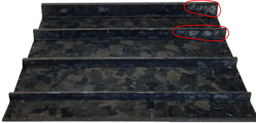
Figure 73: Ribbed surfaces of parts made with short strands under 110 bar with rib-side cooled below 200°C at the thermocouple before flat-side cooling was initiated, highlighting matrix tearing on cooling outlet end of Rib C and Rib D.
