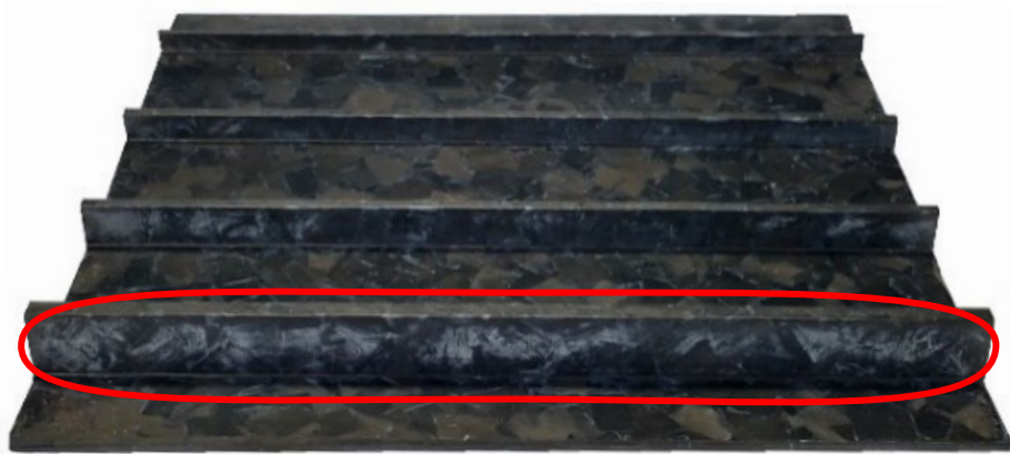
Figure 74: Ribbed surfaces of parts made with short strands under 110 bar with rib-side cooled below 200°C at the thermocouple before flat-side cooling was initiated, highlighting matrix tearing on full side of Rib D.
