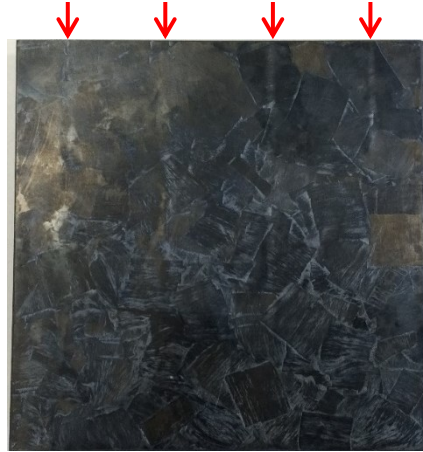
Figure 66: Faint lines visible on the back of the part made with square strands at 30 bar fill pressure and 400°C.
