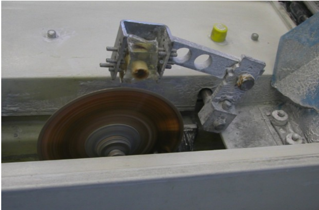
Figure 12. Implant-containing bone embedded in acrylic as it is being sectioned.
