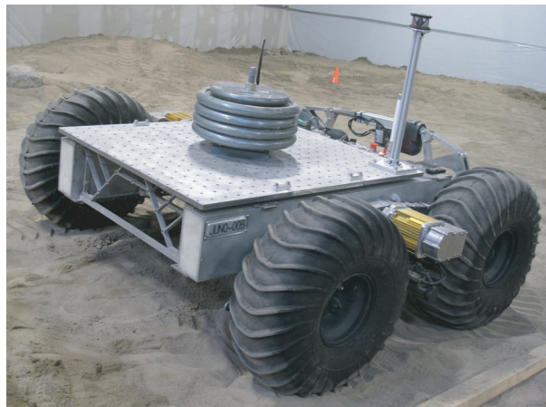
FIGURE 4.21. The rover with the added mass to its main frame.
