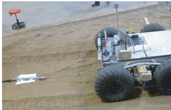
FIGURE 4.10. The descender and the load cell used in the drawbar pull tests
