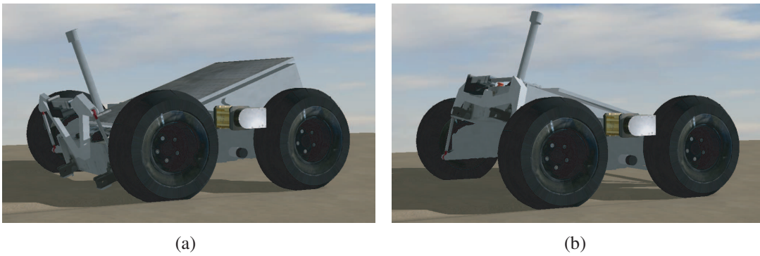
FIGURE 4.4. Simulated Juno rover in Vortex at different tilting configurations.
