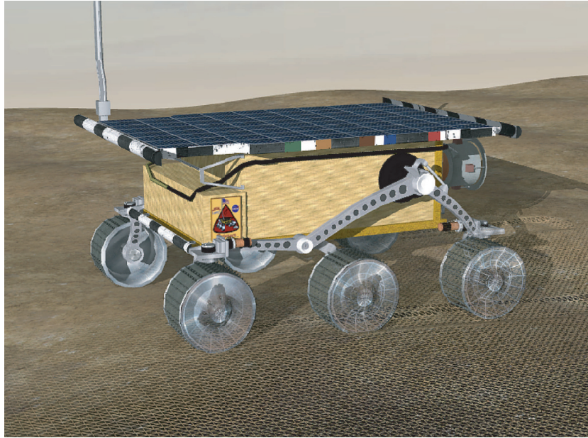
FIGURE 3.31. Sojourner rover simulation in Vortex using the elasto-plasticity model. The rover moves on a height-field and the soil deformation and the hardening parameter are stored in the height-field vertices.
