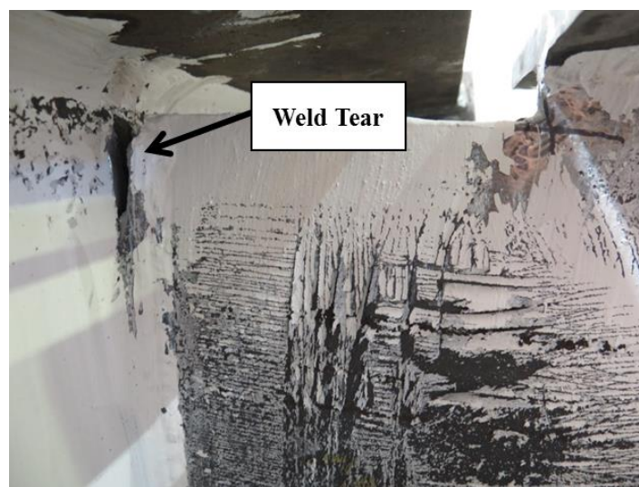
Figure 4.39 – Weld tear in Specimen 10
