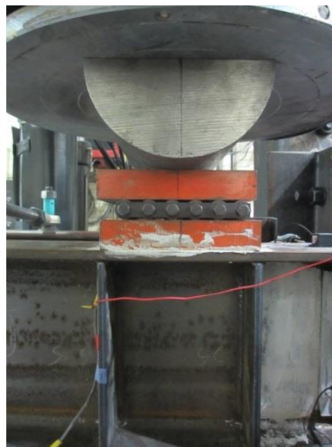
Figure 3.17 – Half cylinder and roller loading system
