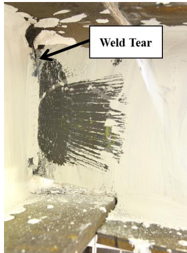
Figure 4.33 – Weld tear in Specimen 8
