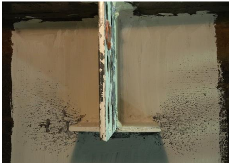
Figure 4.8 – Engagement of girder web due to retrofit plate in Specimen 9J
