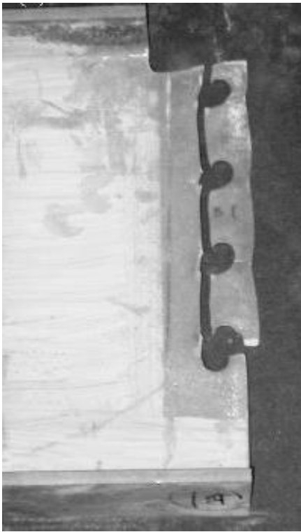
Figure 2.9 – Classical tear-out (Franchuk et al. 2003)
