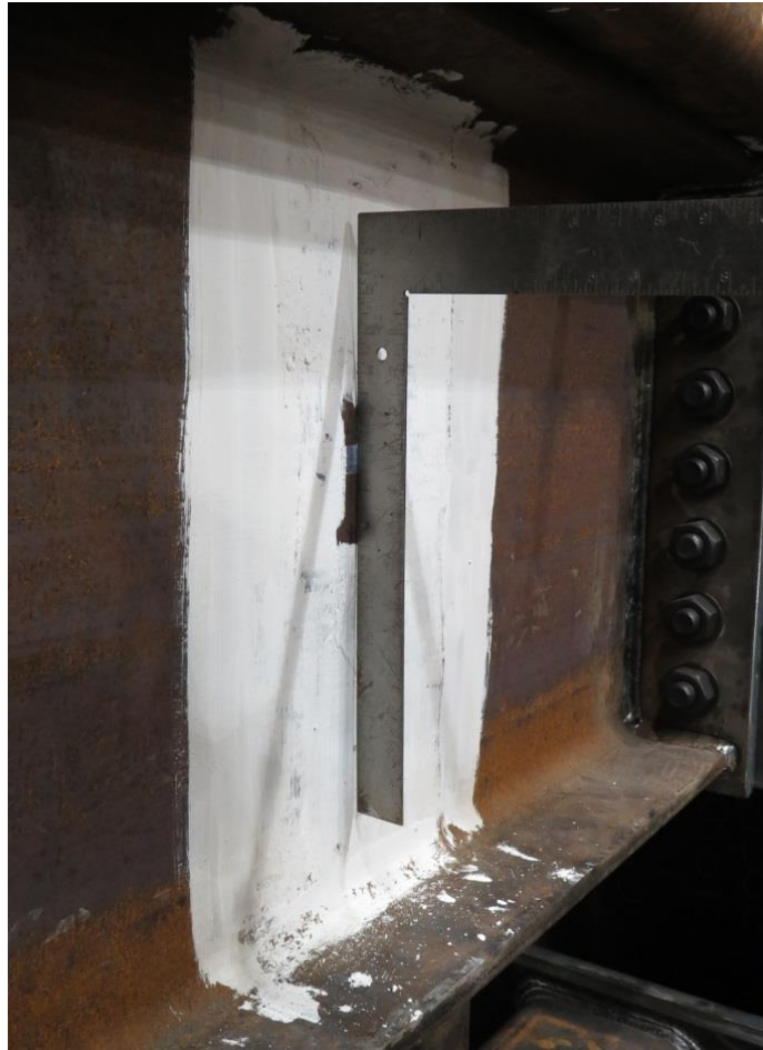
Figure 4.6 – Damage in girder web (girder web punching) in Specimen 6J
