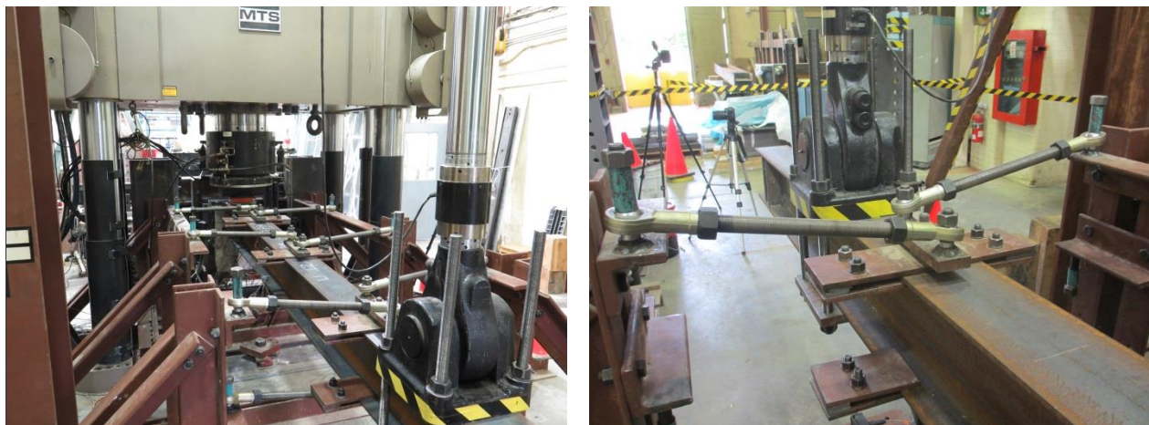
Figure 3.15 – Lateral bracing system: (a) global view; (b) local view
