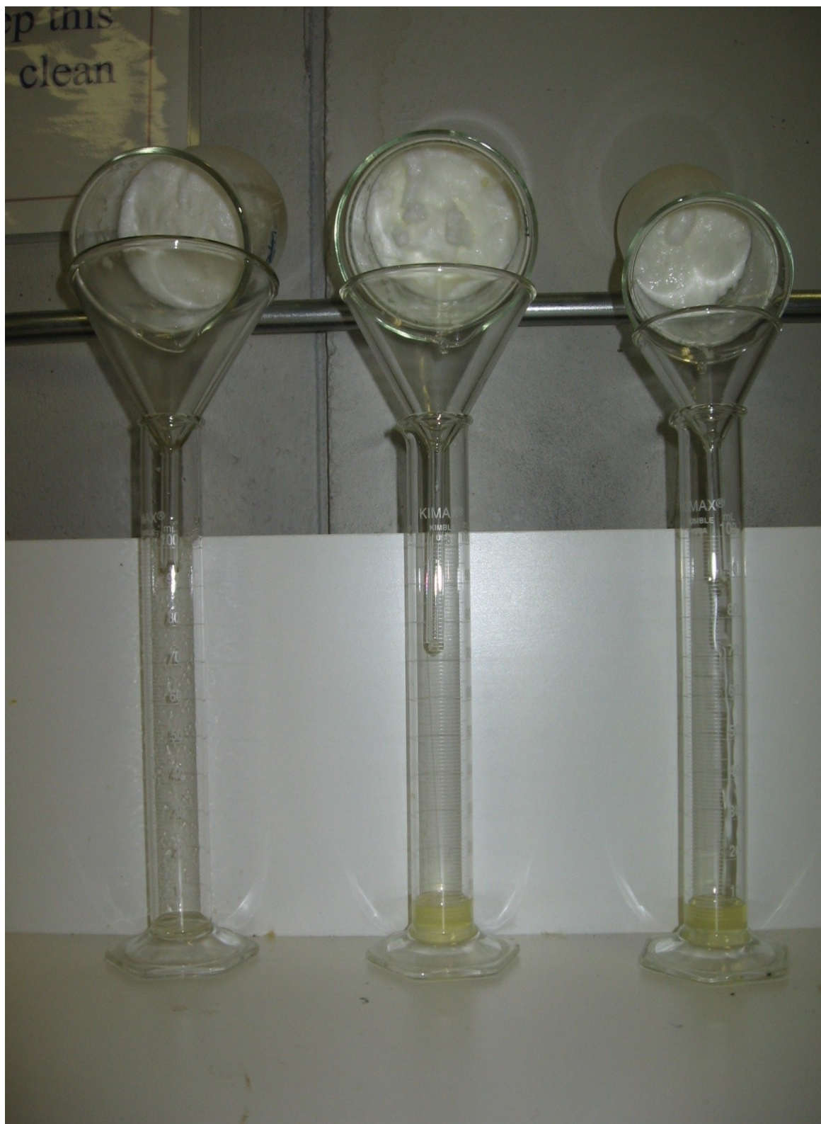
Figure 7.3 Experimental setup for measurement of foam stability
