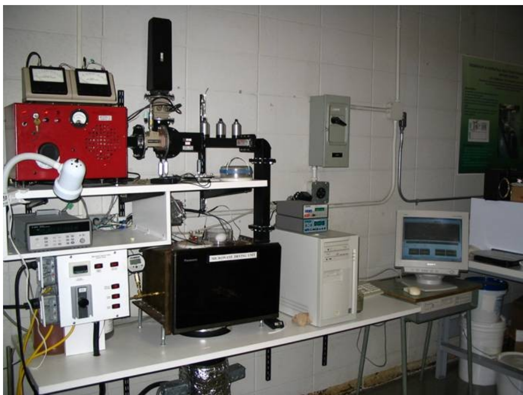
Figure 4.4 Instrumented and computer controlled microwave (MW) oven
