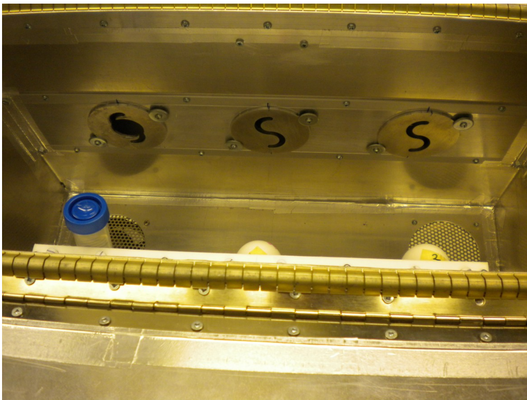
Figure 6.6 S- Parabolic slotted waveguide applicator
