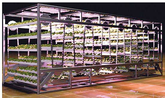
Figure 1 Hydroponic unit with trays and conveyor belt (Urban Barns Inc., 2014)
