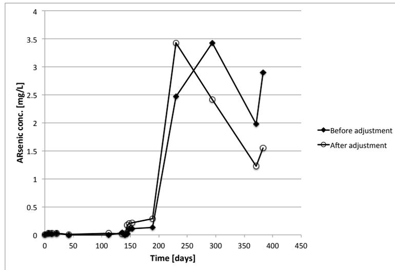
Figure A.12.: Before vs. after adjustment arsenic concentrations as a function of time (CD2b 'Sulfide')
