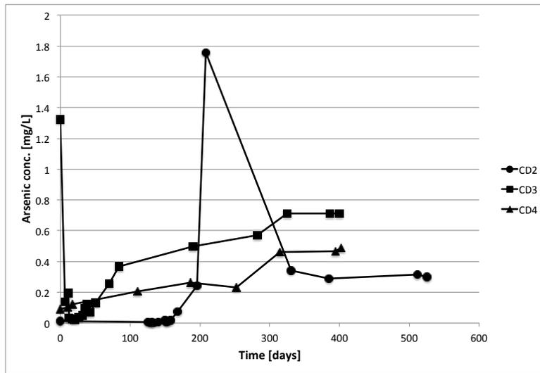
Figure A.14.: NaOH as base: As conc. during Drift stability testing
