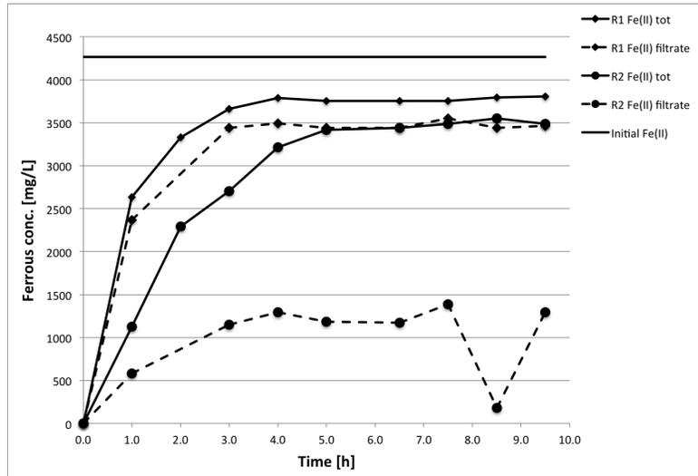
Figure A.1.: CD1 (Fe(II)): Ferrous precipitation in the CCPTN circuit
