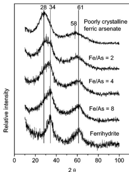
Figure 2.3.: XRD patterns of various co-precipitates compared to ferric arsenate and ferrihydrite with Cu-K $\alpha$  radiation [59]
