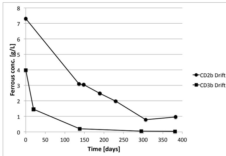
Figure 3.5.: Ferrous concentrations for the 'pH-Drift' series CD2b and CD3b during ageing
