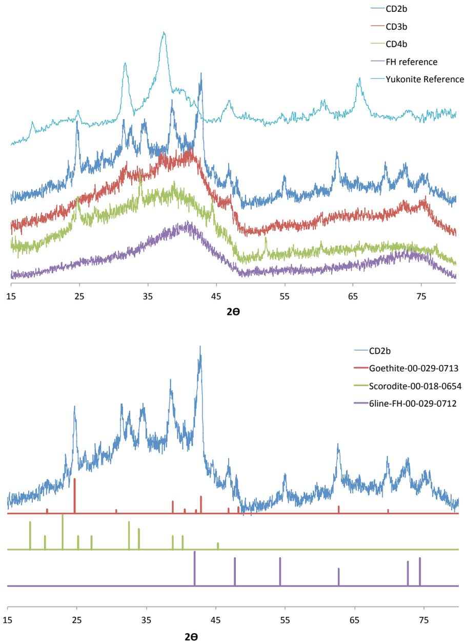
Figure 3.7.: XRD patterns for CD2b/CD3b/CD4b 'Drift' series at termination of experiments vs. ferrihydrite(FH) and yukonite reference (Top) and CD2b 'Drift' series vs. goethite, scorodite and 6line-ferrihydrite (Bottom)
