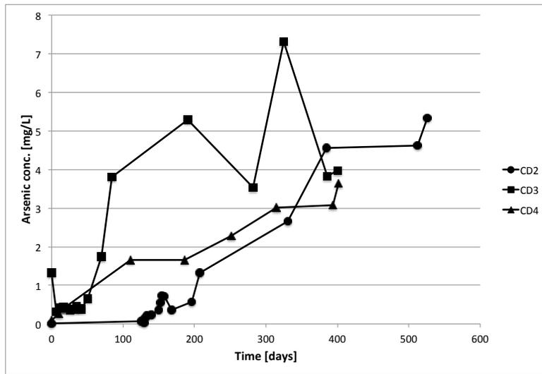
Figure A.16.: NaOH as base: As conc. during Sulfite stability testing
