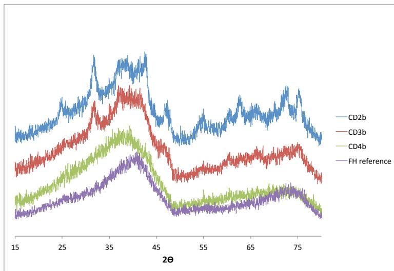
Figure A.8.: XRD patterns for CD2b/CD3b/CD4b 'Oxidic' samples at termination of experiments vs. ferrihydrite reference
