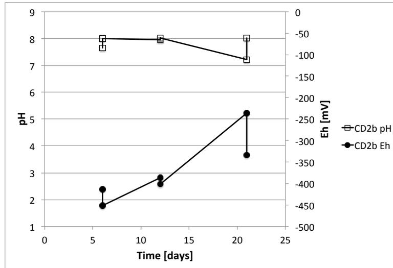
Figure 3.2.: Example for opposite trends in pH-E<sub>h</sub> progression with the used before/after adjustment sampling technique (CD2b 'Oxic')
