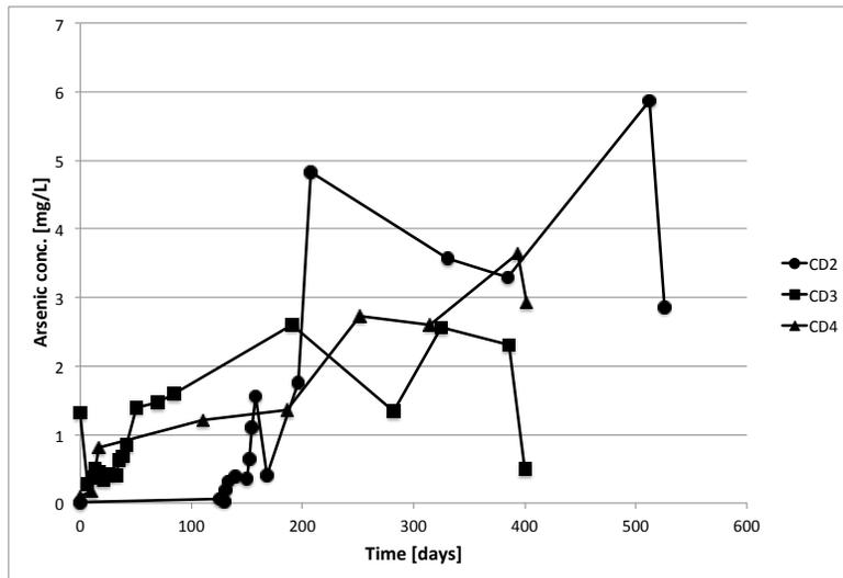
Figure A.17.: NaOH as base: As conc. during Sulfide stability testing
