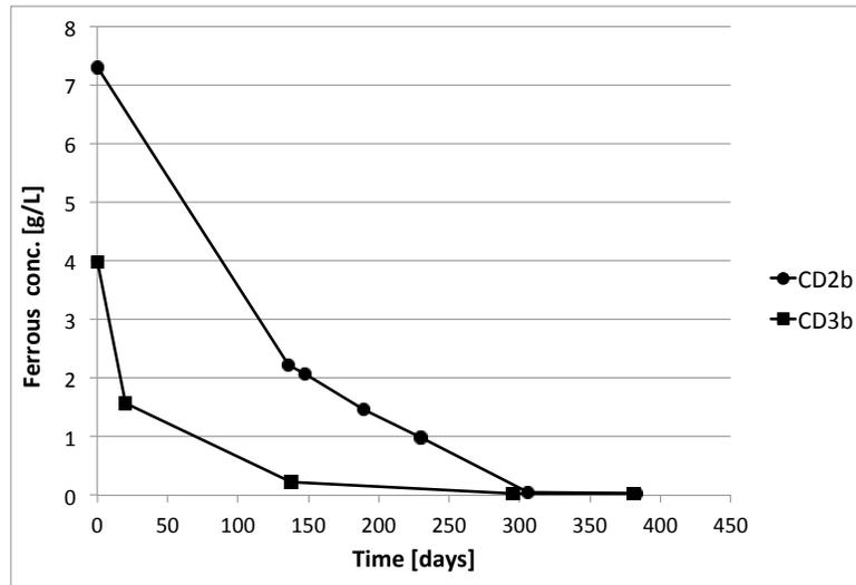
Figure 3.10.: Oxidation of ferrous in CD2b/CD3b 'Oxic' samples
