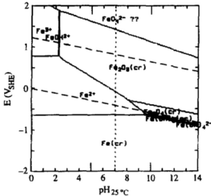
Figure 2.1.: The Fe-H<sub>2</sub>O system at 298K [28]
