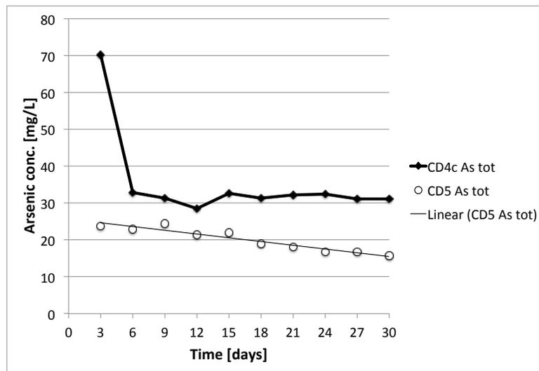
Figure 4.4.: Arsenic concentration release under sulfide-added stability testing of CD4c (Fe(III) / As(V)=4) and CD5 (Fe(III) / Al(III) / As(V)=2/2/1)
