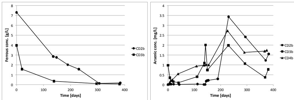
Figure 3.14.: The oxidation of Fe(II) for all 'Sulfide' samples (Left) and the arsenic concentrations during stability testing for all 'Sulfide' samples (Right)
