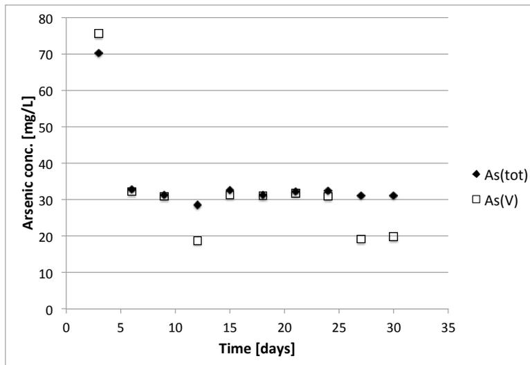
Figure 4.5.: Arsenic speciation data (As(tot) and As(V)) for CD4c (Fe(III) / As(V)=4) under sulfide-added anoxic stability testing
