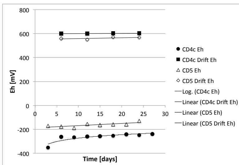
Figure 4.2.:  $E_h$  progression for CD4c (Fe(III) / As(V)=4) and CD5 (Fe(III) / Al(III) / As(V) = 2 / 2 / 1) during anoxic stability testing with and without sulfide reagent addition
