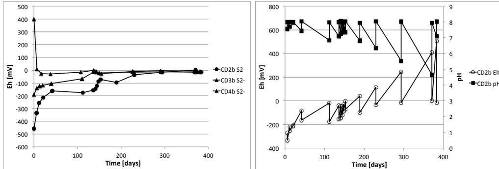
Figure 3.13.: E<sub>h</sub> progression for all 'Sulfide' after-adjustment samples in mV (Left) and E<sub>h</sub>-pH progression before and after adjustment for CD2b S<sub>2</sub><sup>-</sup> (Right)
