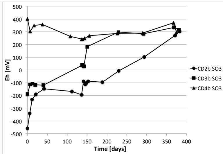
Figure 3.11.:  $E_h$  progression for all 'Sulfite' samples after-adjustment samples in mV
