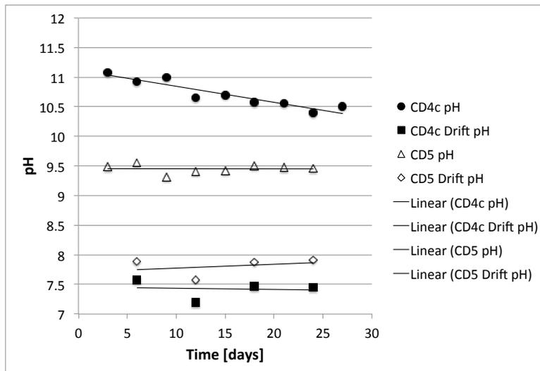
Figure 4.1.: pH progression for CD4c (Fe(III) / As(V)=4) and CD5 (Fe(III) / Al(III) / As(V)=2/2/1) during anoxic stability testing with and without added sulfide reagent
