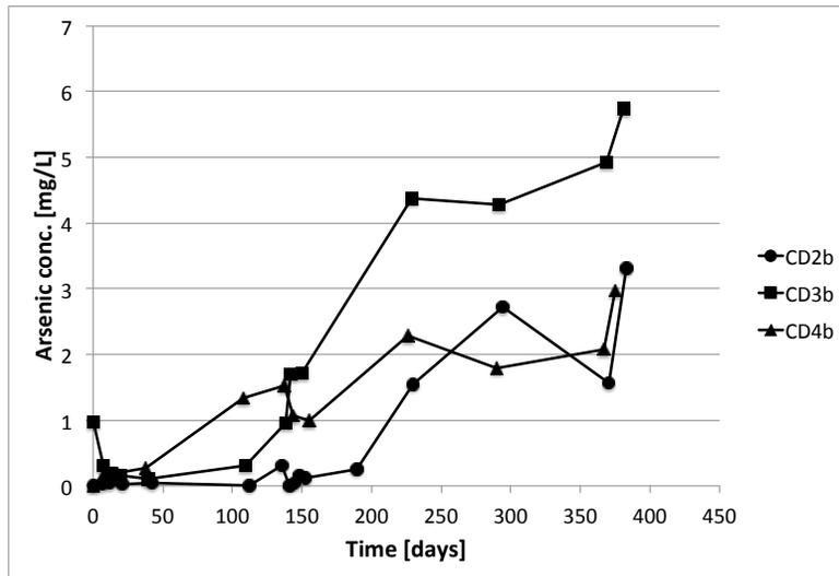
Figure 3.12.: Arsenic concentration for the 'Sulfite' samples during long-term stability testing
