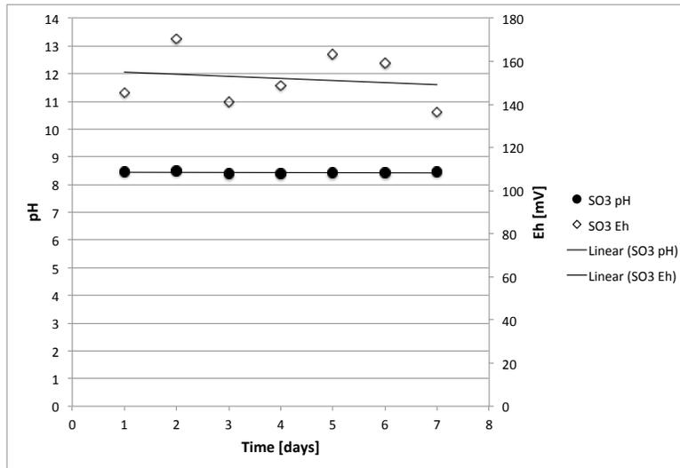
Figure A.20.: pH and  $E_h$  progression for CD4c (Fe(III)/As(V)=4) under excess  $\text{SO}_3^{2-}$ -added stability testing
