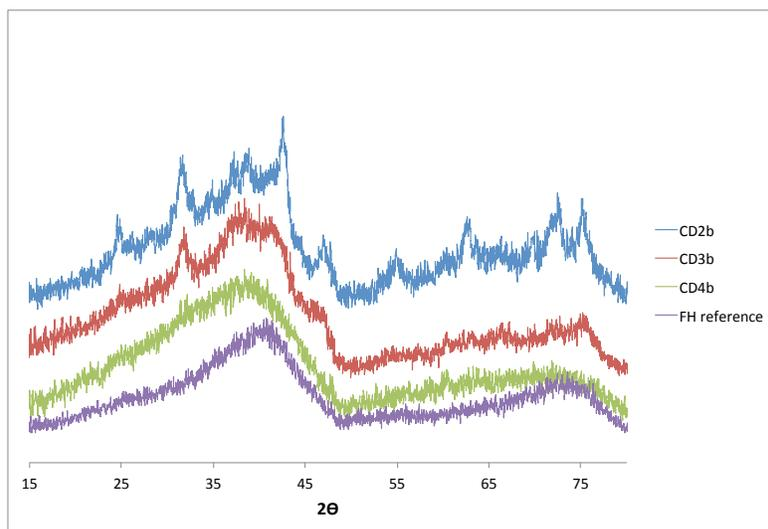
Figure A.10.: XRD patterns for CD2b/CD3b/CD4b 'Sulfite' samples at termination of experiments vs. ferrihydrite reference
