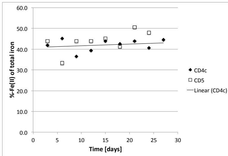
Figure 4.3.: Percentage of total iron as ferrous for CD4c (Fe(III) / As(V)=4) and CD5 (Fe(III) / Al(III) / As(V)=2/2/1) during sulfide-added anoxic stability testing
