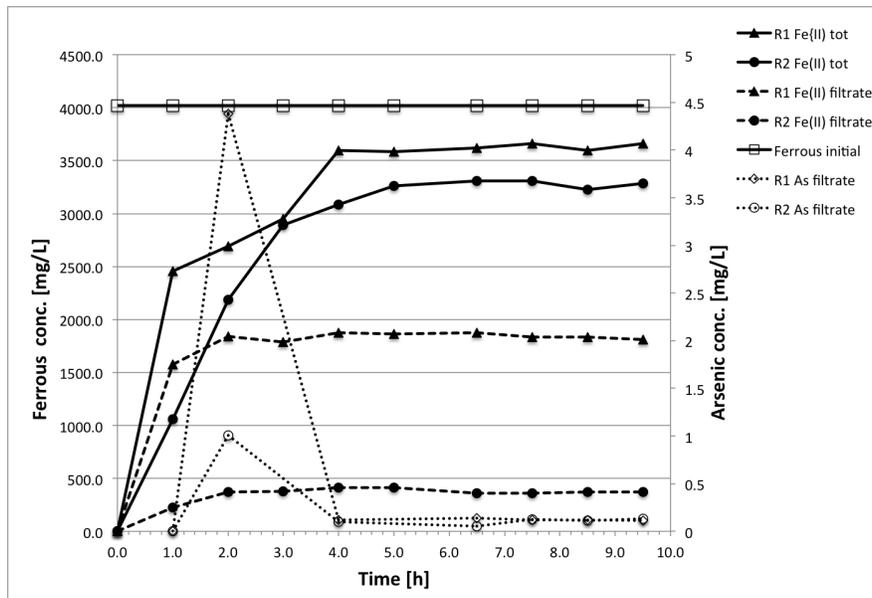
Figure 3.3.: CD2 (Fe(II)/As(V)=4): Ferrous and arsenic concentration profiles during co-precipitation
