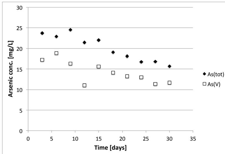
Figure 4.6.: Arsenic speciation data (As(tot) and As(V)) for CD5 (Fe(III) / Al(III) / As(V)=2/2/1) under sulfide-added anoxic stability testing
