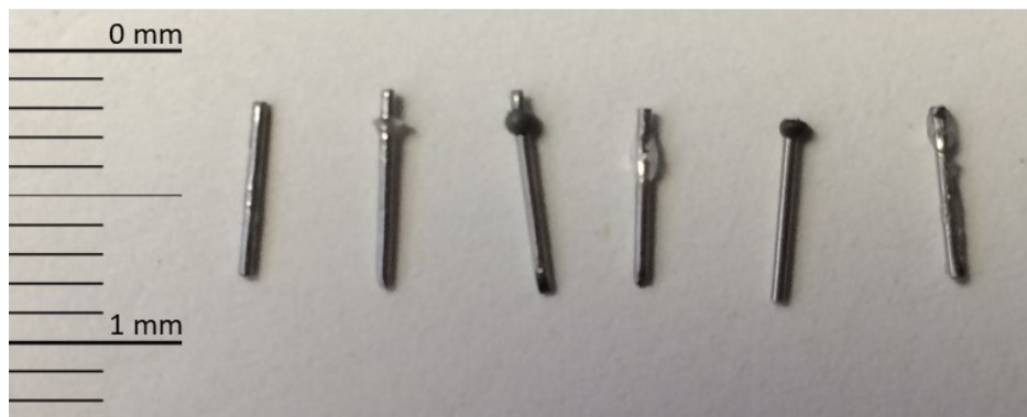
FIGURE 3.7: Image of the \sim 6 mm needles with different blobs. Blobs are made from instant adhesive or cold-weld-two-part epoxy, and are placed at the end or offset from the end of the needle. From left to right the blobs material-location are: no-blob (standard needle), adhesive-offset, epoxy-offset, adhesive-offset, epoxy-end, and adhesive-end.
