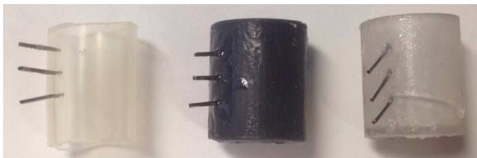
FIGURE 3.8: Image of the three combinations of core-material and needle attachment, which achieved watertightness and allowed needle rotation between 0^\circ and 60^\circ . From left to right: silicone rubber tube with tight-fit needles, flexible photopolymer with glued needles, and polycarbonate tubing with needles on silicone rubber hinges.
