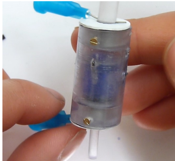
FIGURE 3.13: Image of the finished capsule assembly. The capsule is filled with water, used for the prototype test, and tinted blue, to facilitate its visualization.
