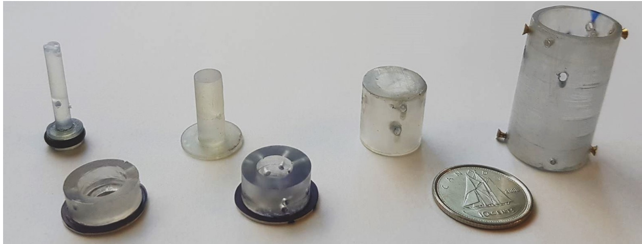
FIGURE 3.12: Image of the capsule components. From left to right: piston, deployment cap, retraction pusher, retraction cap, core (with sleeve), and case. These components were assembled to build the complete capsule.
