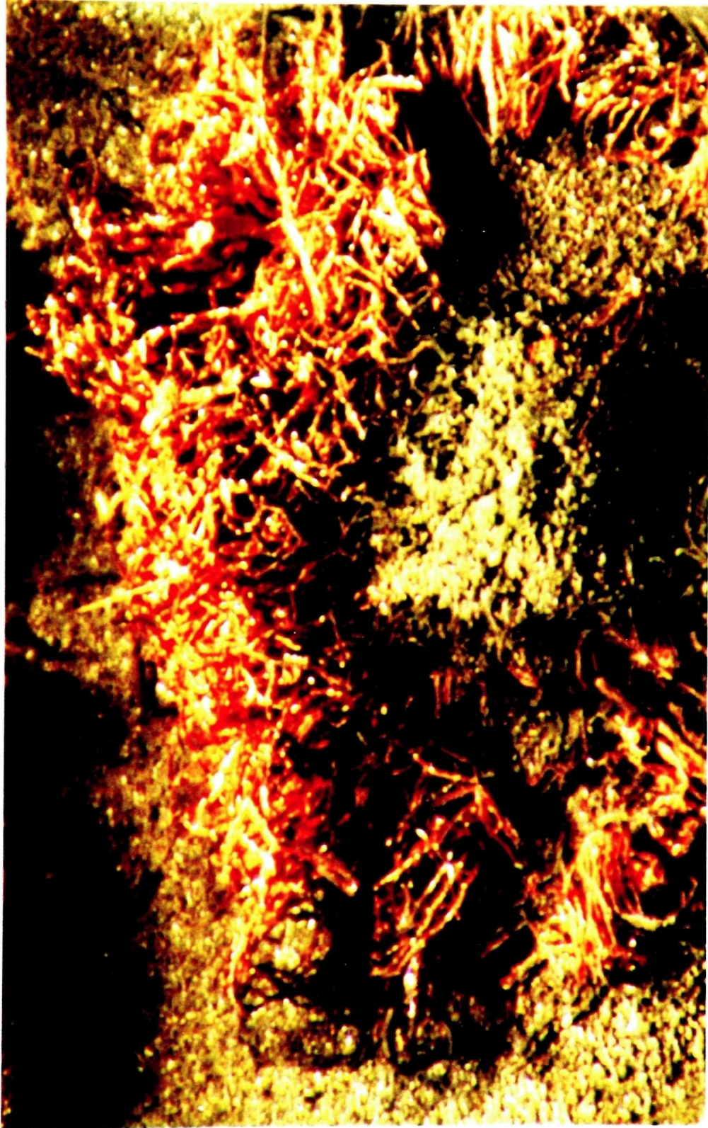
Figure 3.10. Copper fibres with a diameter of about 30\text{ }\mu\text{m} , precipitated at the last surface to freeze of the excess copper ingot DH-B10.
