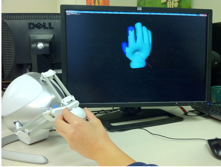
Figure 1–1: Our haptic simulation framework: The 3D hand model is deformed in an interactive simulation using the 3-DOF Novint Falcon haptic device.
