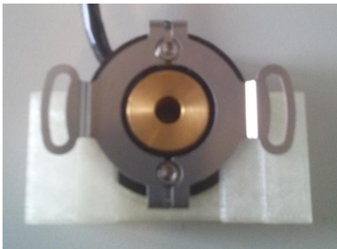
Figure 13: Initial 3D print of mount for optical encoder, shown with encoder
