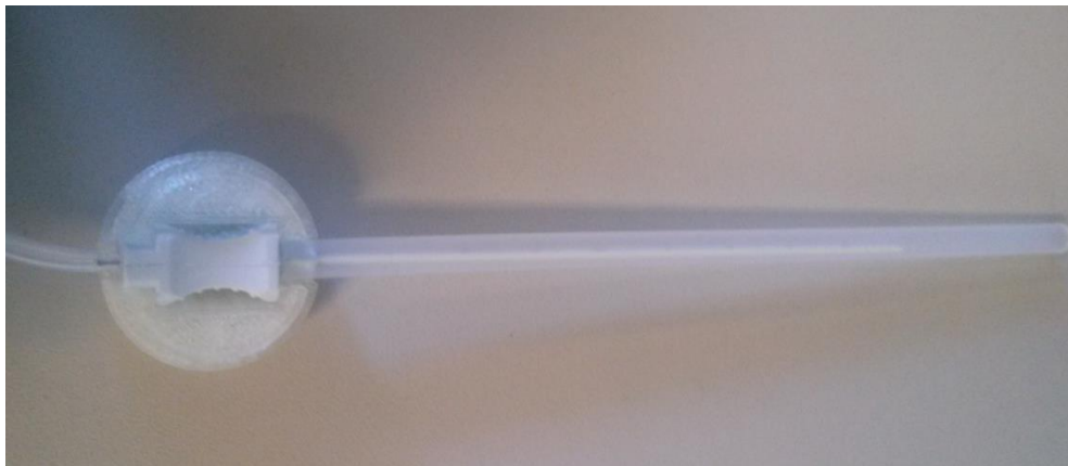
Figure 11: Initial clamp design for 21G insulated peripheral nerve block needle
