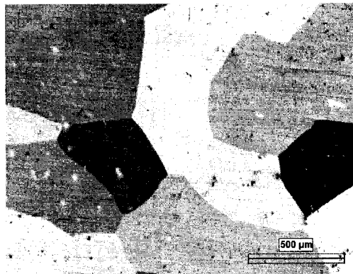
Figure 3.1 – Optical micrograph of the FA-129 intermetallic microstructure.
