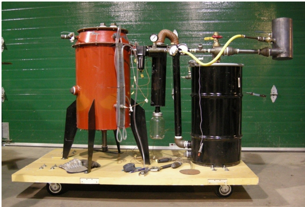
Figure 1.1 – Photograph of the GEK gasifier used for experiments on CO 2 enrichment from biomass
