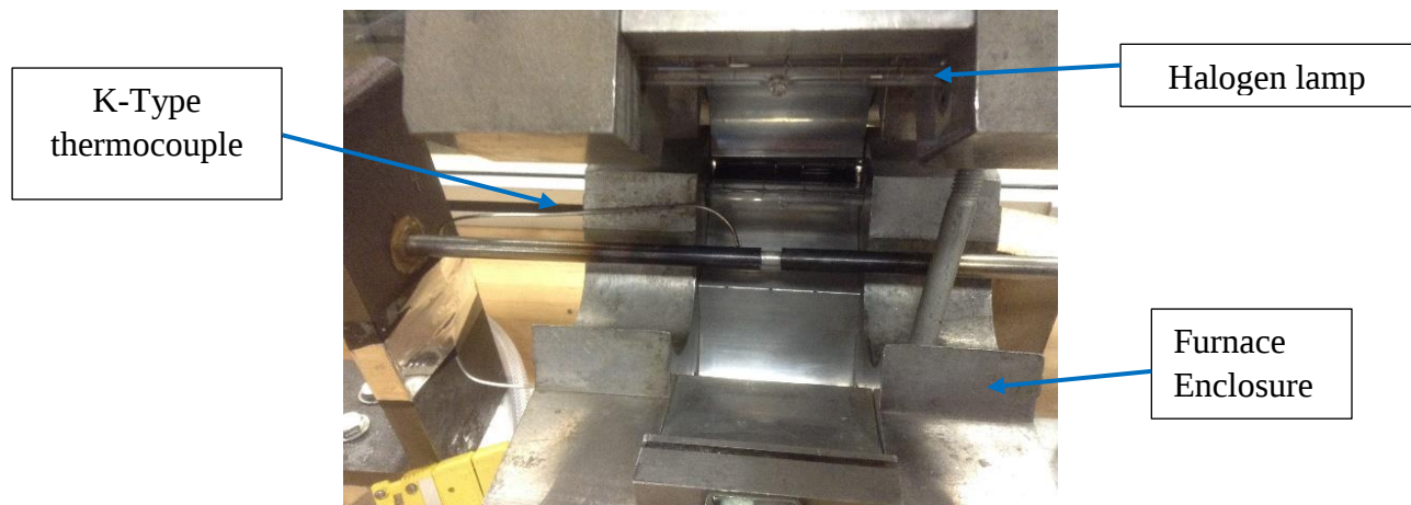
Figure 3.6. Radiative furnace placement at bars-sample interface.
