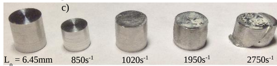
Figure 4.2. Strain rate sensitivity results of AA7050-T7451 at 25°C. a) True stress vs true strain. b) True strain vs strain rate. c) Deformed sample from varying strain rate tests.
