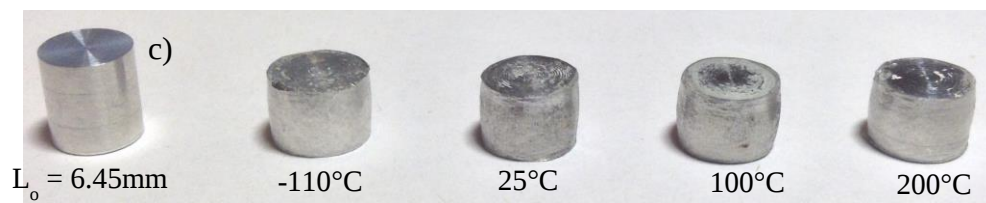
Figure 4.4. Temperature sensitivity results of AA7050-T7451 at a nominal strain rate of 2000 s^{-1} . a) True stress vs true strain. b) Strain rate vs true strain. c) Deformed samples from varying temperature tests.
