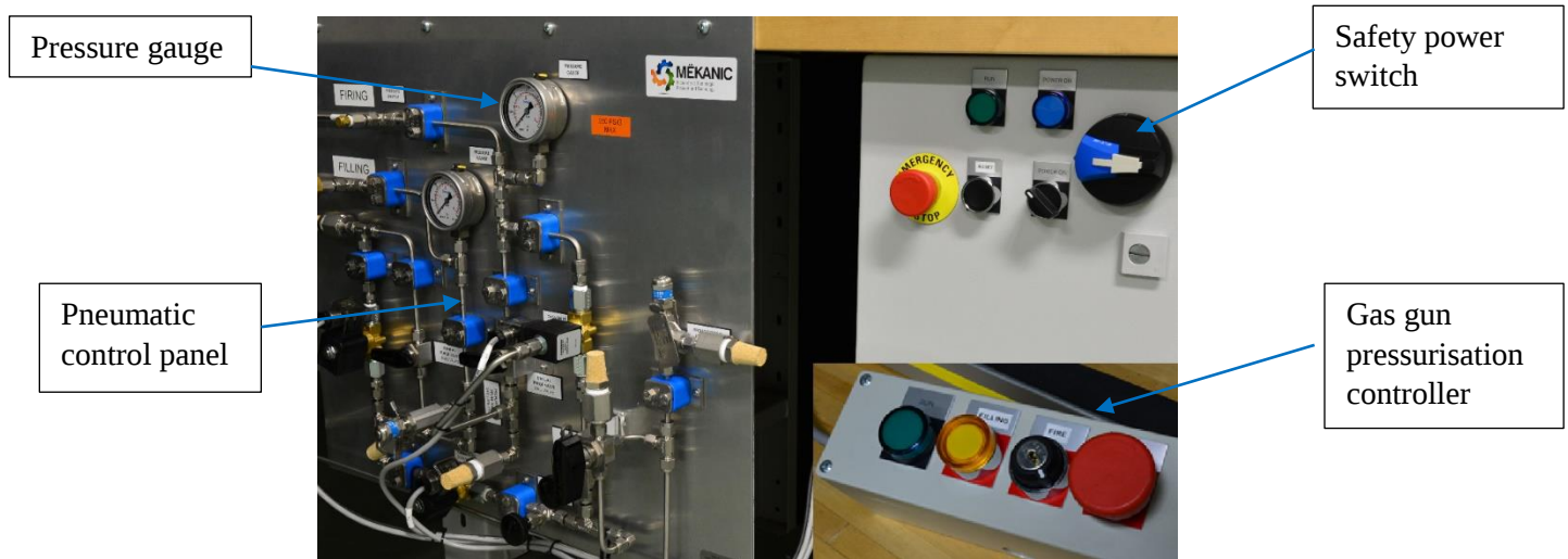
Figure 3.2. Pneumatic control panel and gas gun pressurisation controller.
