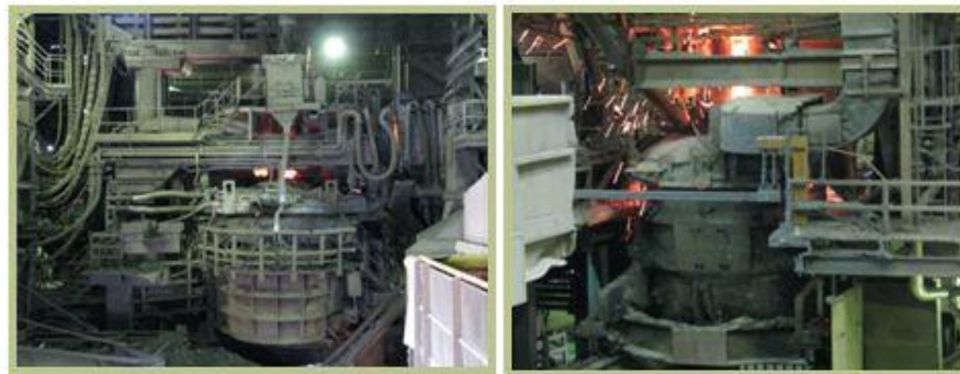
Figure 4: Melting process at Electric Arc Furnace
