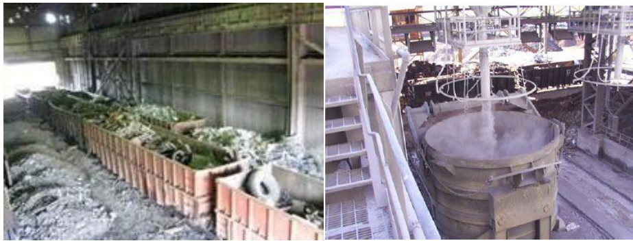
Figure 2: Scrap loading bay and scrap bucket at Arcelormittal Contrecoeur
