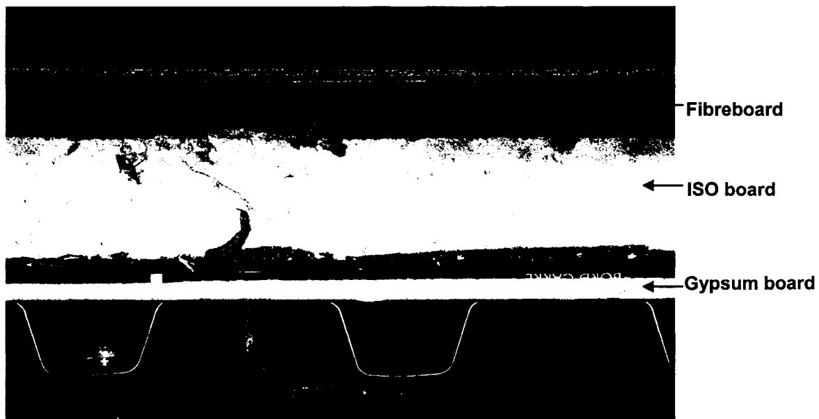
Figure 2.1: Roof cross-section tested by Yang (2003)
