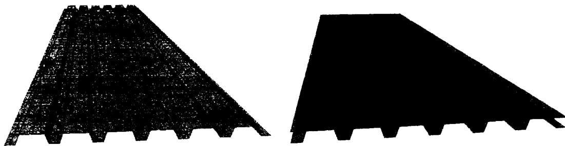
Figure 2.2: Underformed shapes of bare sheet steel deck (left) and deck with gypsum elements (right) (Yang, 2003).
