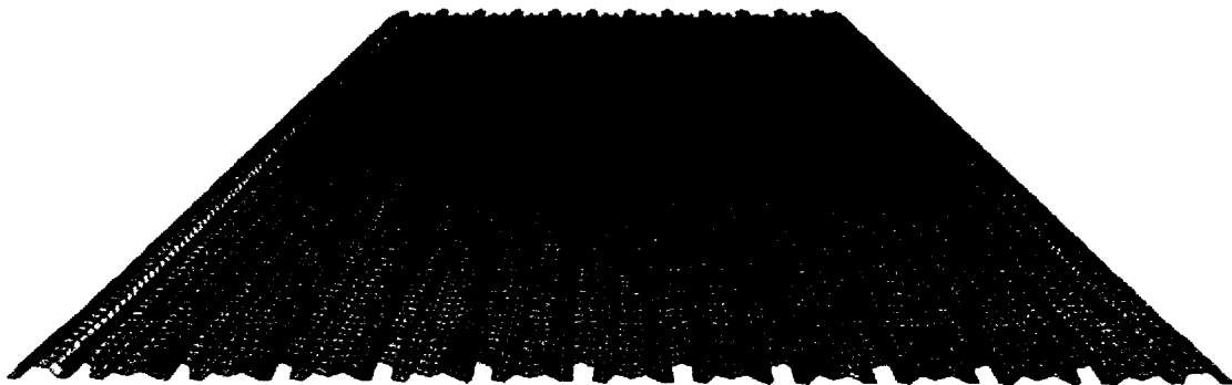
Figure 4.29: Deformed shape of bare steel deck
