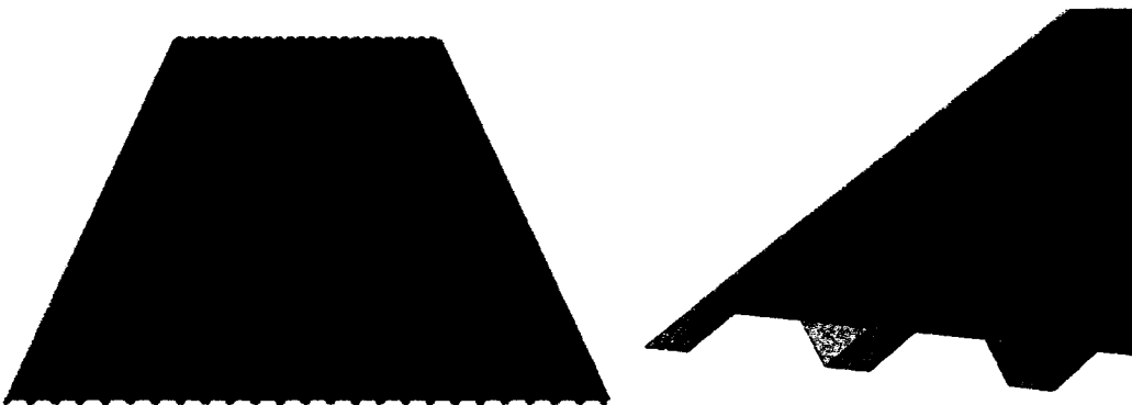
Figure 4.24: Undeformed shape of full-scale steel deck model with roofing elements
