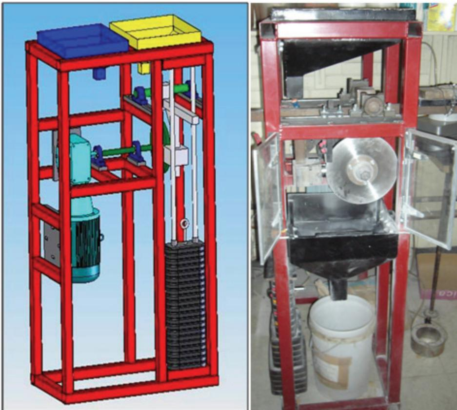
Figure 3-1: SWAT apparatus, Version 3 (left) CAD design, (right) apparatus
