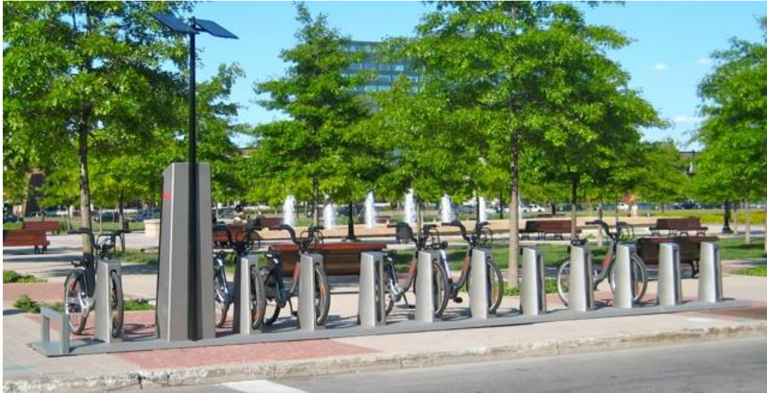
Figure 11. BIXI's solar-powered, modular station. Source: Ratthé, 2009.
