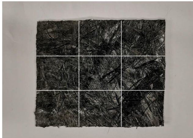
Figure 4.6 Thicknesses of the nine areas to be measured
