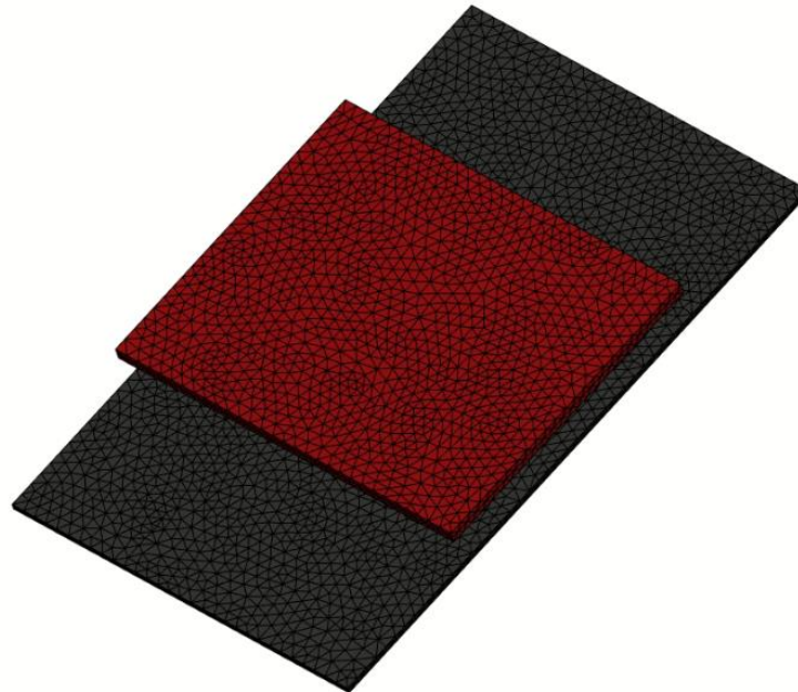
Figure 5.3 The meshed charge and part
