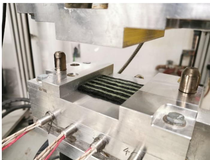
Figure 4.1 One-dimensional flow-compaction test
