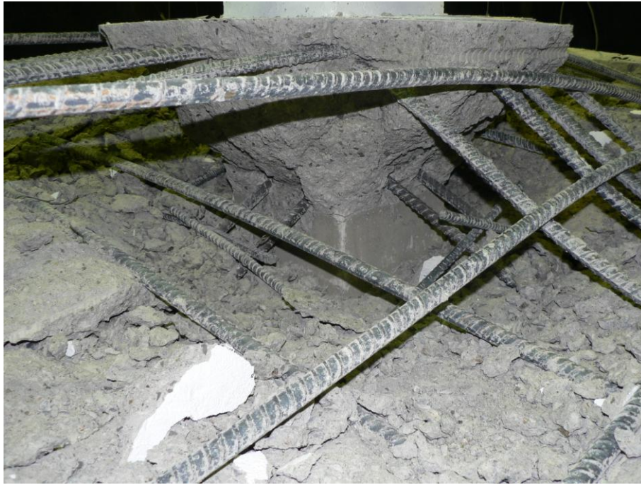
Fig. 4.31. Inclination of structural integrity reinforcement after testing completed (specimen D1)
