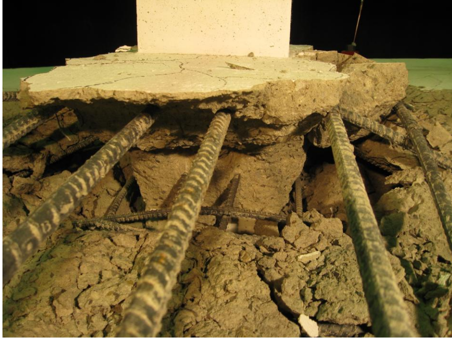
Fig. 4.43. Inclination of structural integrity reinforcement at end of testing with 10M bars breaking out of the bottom surface of the punching cone (specimen D2)
