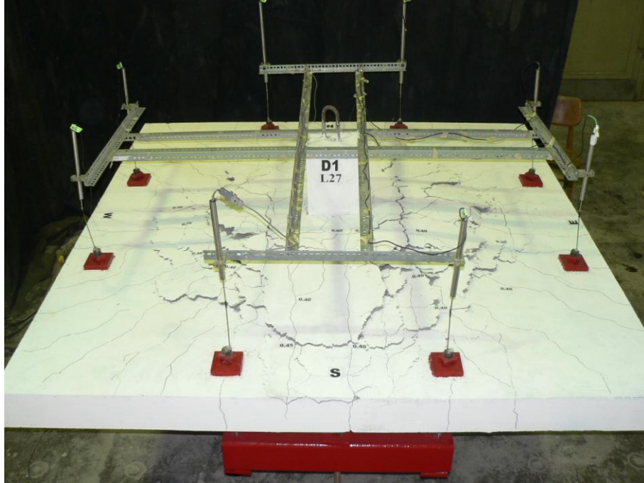
Fig. 4.29 Ripping out of top mat of reinforcement at a displacement of 75mm (specimen D1)
