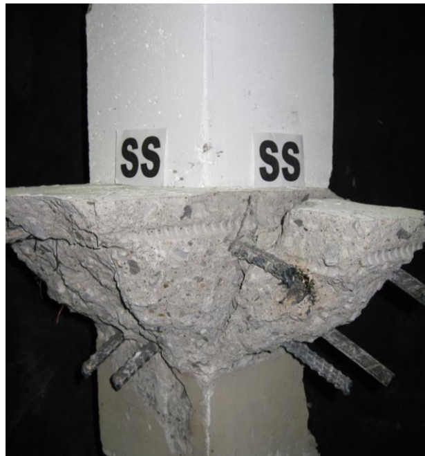
Fig. 4.8. Integrity reinforcing bars after slab removal (specimen SS)
