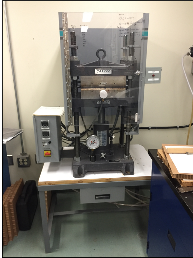
Figure 4.3 – Hot-press molding machine (Carver Manual Hydraulic Press with Watlow Temperature Controllers, Model #3856, Carver Inc.).
