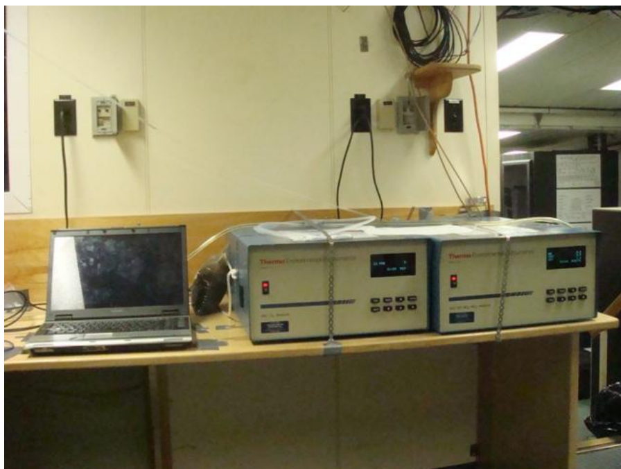
Figure 3A. Ozone and Nox analyzers in CCGS Hudson during Labrador Mission 2009
