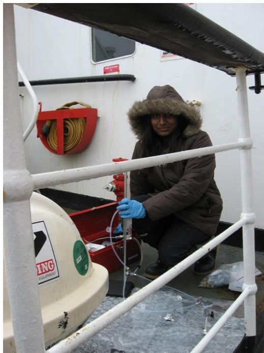
Figure 7b Collection of marine air in Teflon bag on Hudson during the Labrador mission 2009
