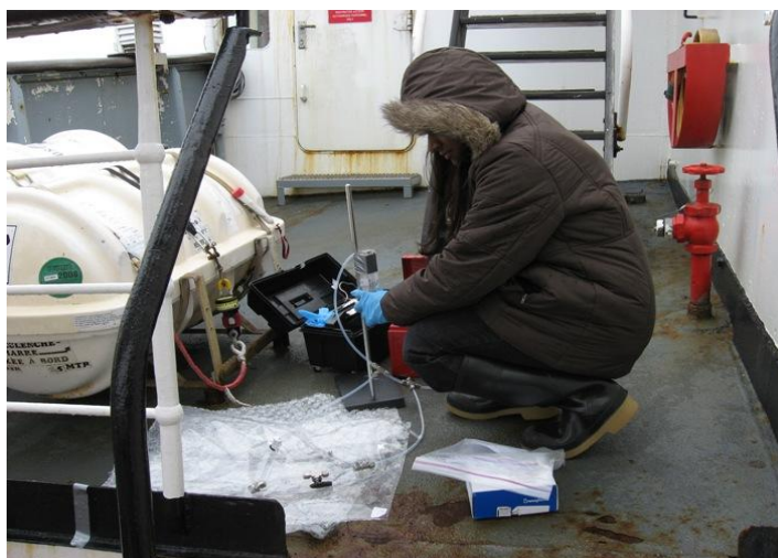
Figure 7a Collection of marine air in Teflon bag on Hudson during the Labrador mission 2009
