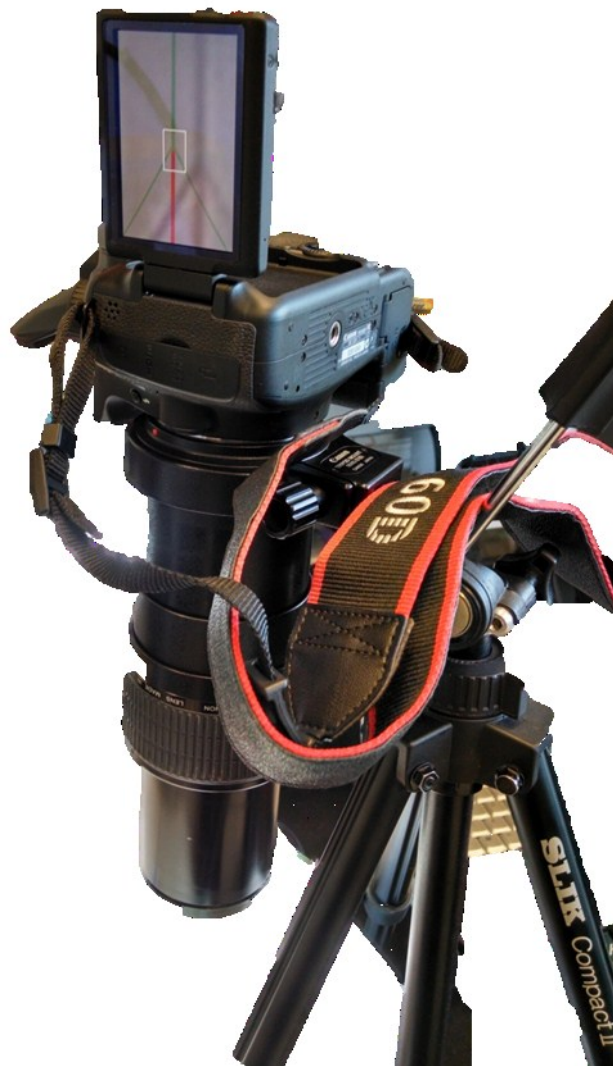
Fig. A2: Camera setup for flow visualization using food dyes within microfluidic device.
