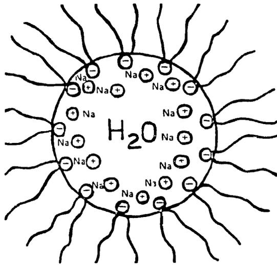
FIGURE 1-3 - Structure of AOT reverse-micelle
