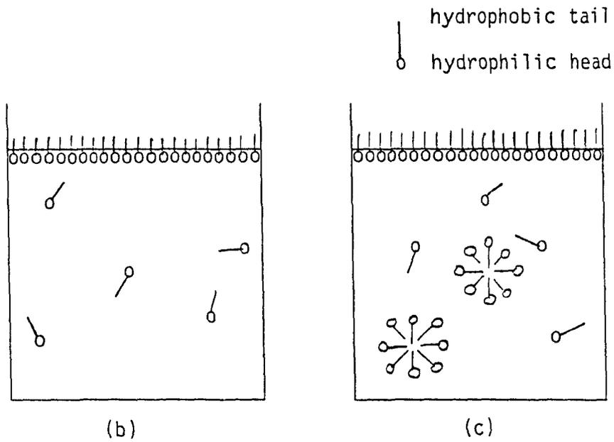
FIGURE 1-2 - Surface tension and micelle formation
