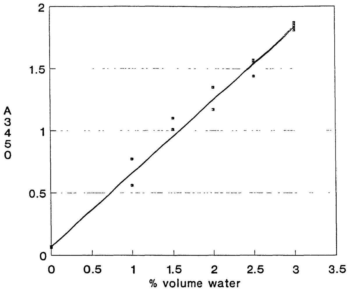
FIGURE 4-2 - IR calibration curve for water
