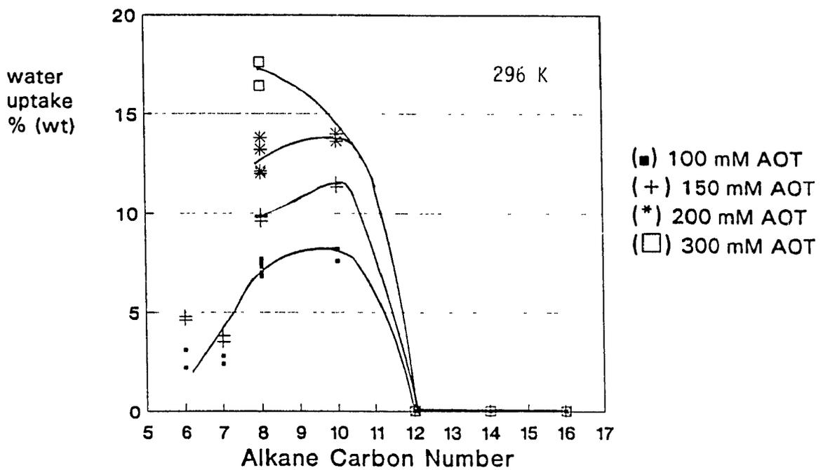
FIGURE 5-2B - Effect of alkane carbon number on water uptake for AOT
