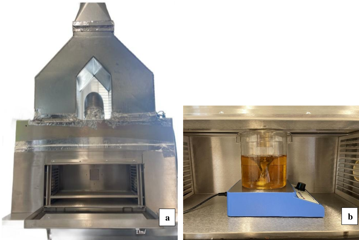
Figure 4.1. Pulsed light treatment system: (a) SteriPulse-XL RS-3000C and mixing setup (b).
