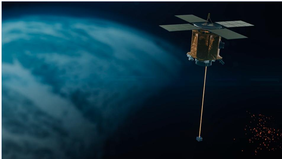
**Figure 1.3:** Tethered space debris removal system [15]
