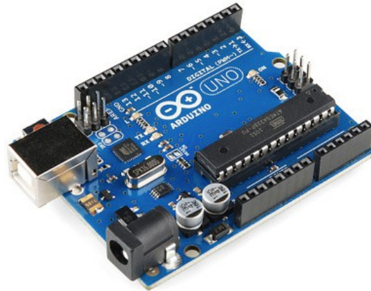
Figure 4.21: Arduino Uno micro-controller board (Source: http://www.arduino.cc , retrieved 2012 June 1)
