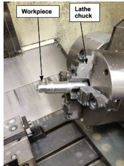
Figure 4.17: Photograph of the workpiece mounted in the chuck (stationary) between lathe operations. The chuck is tilted to facilitate the mounting process and is untilted during machining.
