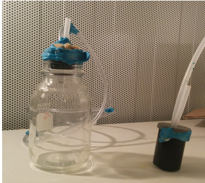
Figure 4.28: Glass bottle (left) and film canister (right) used as buffer volumes in this study. Only one buffer volume is connected to the middle-ear cavity in each experiment.
