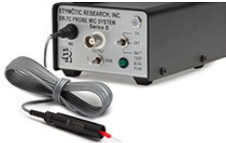
Figure 4.6: ER-7C probe microphone system. (Source: http://www.etymotic.com/pro/er7c-acc.aspx , retrieved 2013 May 30)
