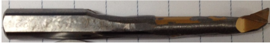
Figure 4.18: Boring tool used to remove material from the inside surface of the coupler.
