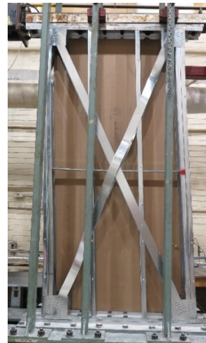
Figure 3.4 Yielding of the straps in tension and buckling of the straps in compression
