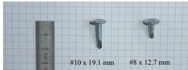
Figure 2.18 Self-drilling wafer head screws used in the specimens (scale in cm)
