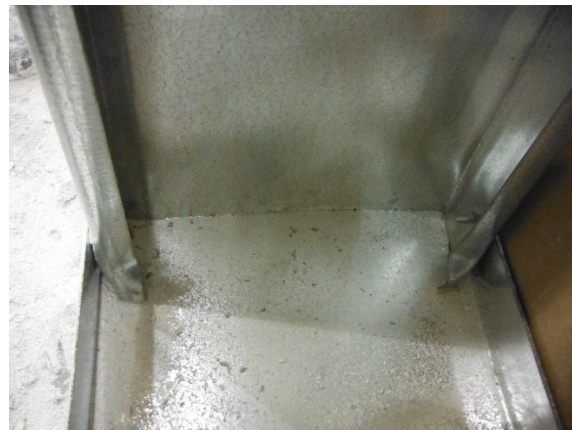
Figure 3.2 Interior stud lip local buckling
