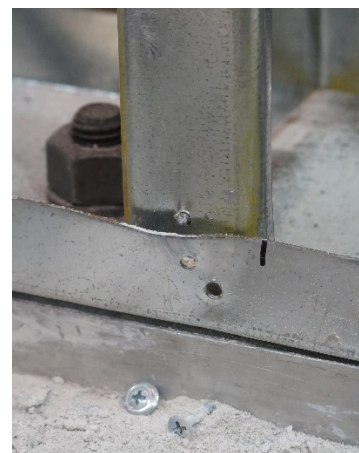
Figure 3.6 Shear failure of the screw
