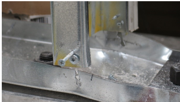
Figure 3.5 Bearing failure of the flanges of the track and localized damage of the track
