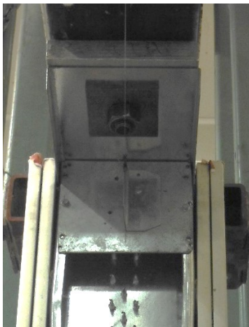
Figure 2.24 String potentiometer installed on the top south of the wall
