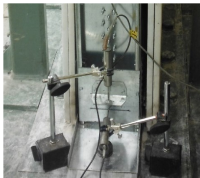
Figure 2.25 LVDTs set up at the south corner of the wall
