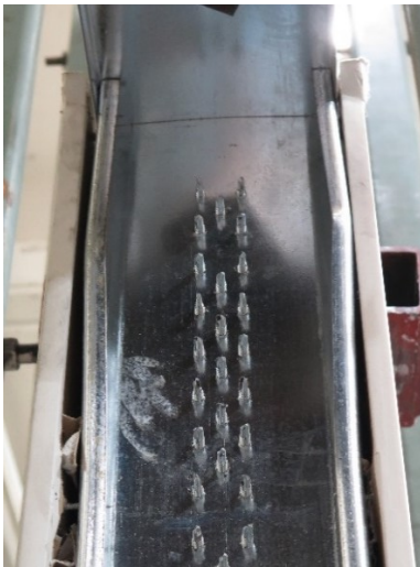
Figure 3.3 Chord stud flange distortional buckling
