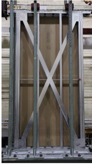
Figure 2.1 Strap-braced gypsum-sheathed shear wall in the test frame
