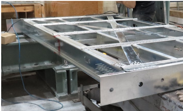
Figure 2.22 Resilient channels installed on the frame
