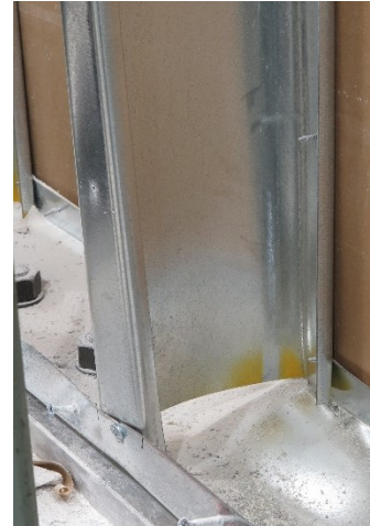
Figure 3.8 Section distortion of the interior studs
