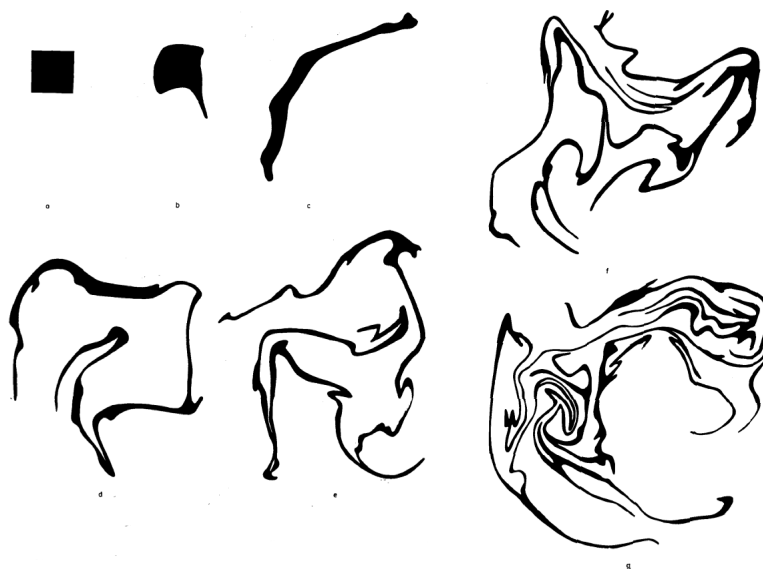
Figure 1–1: Deformation of a fluid element as observed by Welander ( Welander , 1955) in a film of butanol over water. The size of the tank is 50 \times 30 \times 30 cm. The flow is lamellar and the tank is rotating to keep the motion two dimensional.
