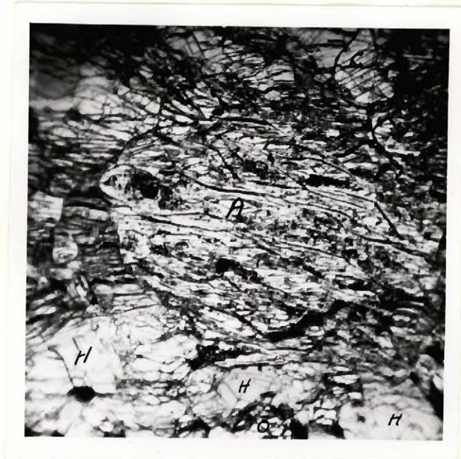
Fig.19 Section of peridotite from a surface sample The olivine has altered to antigorite(A) the opaque material is magnetite, note twinned crystal of calcite (C) in upper right corner, hornblende (H) borders antigorite at the bottom of the section.
