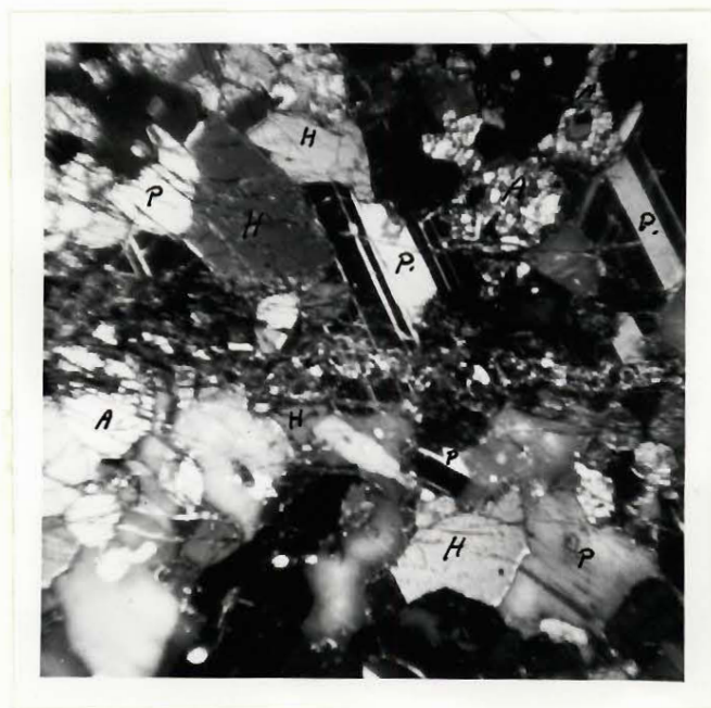
Fig.16 Gabbro under crossed nicols, note hornblende (H), and plagioclase laths (P) offset by a fracture which is now filled with quartz, augite (A) encloses plagioclase.
