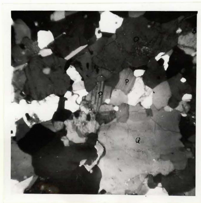
Fig.7 Quartz - biotite - feldspar gneiss under crossed nicols, note strained quartz (Q) and albite twinned plagioclase (P) (X36)
