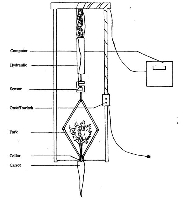
A.IV. Carrot pulling apparatus. Carrot is placed in stationary collar at the junction of petiole and crown. A fork attached to a hydraulic is clamped onto petioles as close to the crown as possible. The hydraulic is turned on and pulls the fork upwards. A sensor on the "s" shaped metal object records to a computer the amount of force (Newton per square meter = Pa) required to pull petioles from the root.
