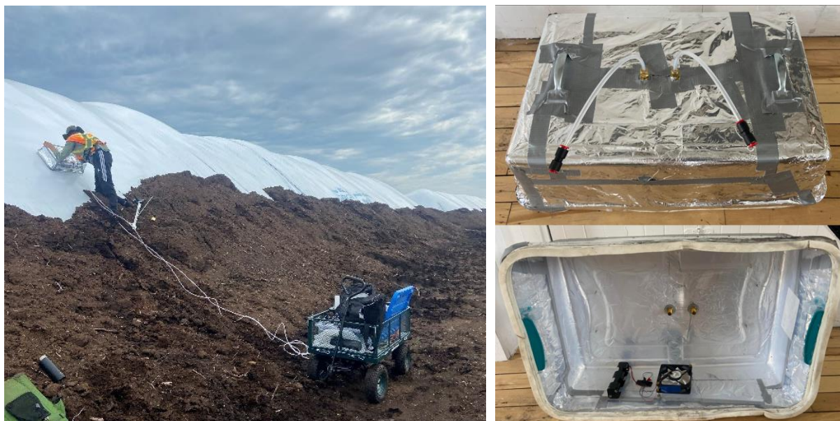
Figure 3.10: Left: flux measurement on covered stockpile, and right: chamber used for flux measurements on covered stockpiles.
