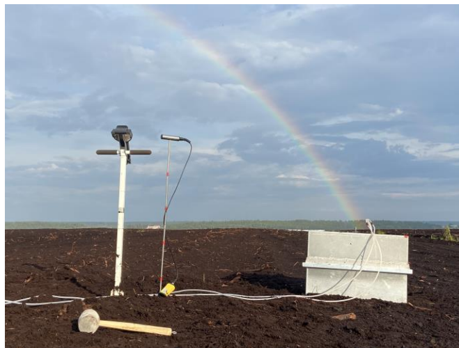
Figure 3.6a: Field equipment used in field operations data collection (left probe: HydroSense II Handheld Soil Moisture Sensor, right probe: Greisinger G1791 Soil/Compost Thermometer, collar-chamber structure, & rubber mallet).
