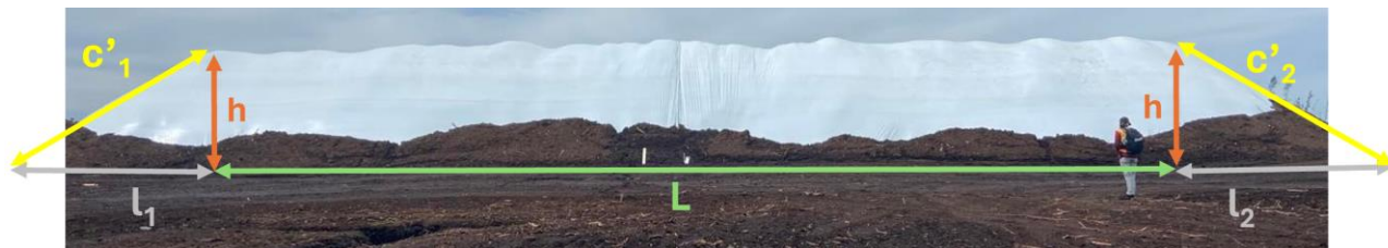
Figure 3.15a: Geometric shapes used to estimate surface area of stockpiles. Left: triangular prism used to represent the main body of a stockpile, and right: oblique pyramid used to describe both ends of a stockpile. Image source: www.khanacademy.org .
