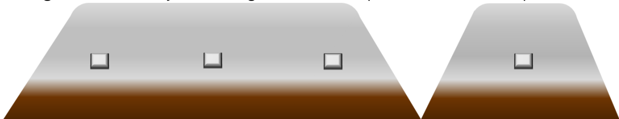
Figure 3.9b: Side view of flux measurement positions on the long (left) and short (right) faces of covered stockpiles.
