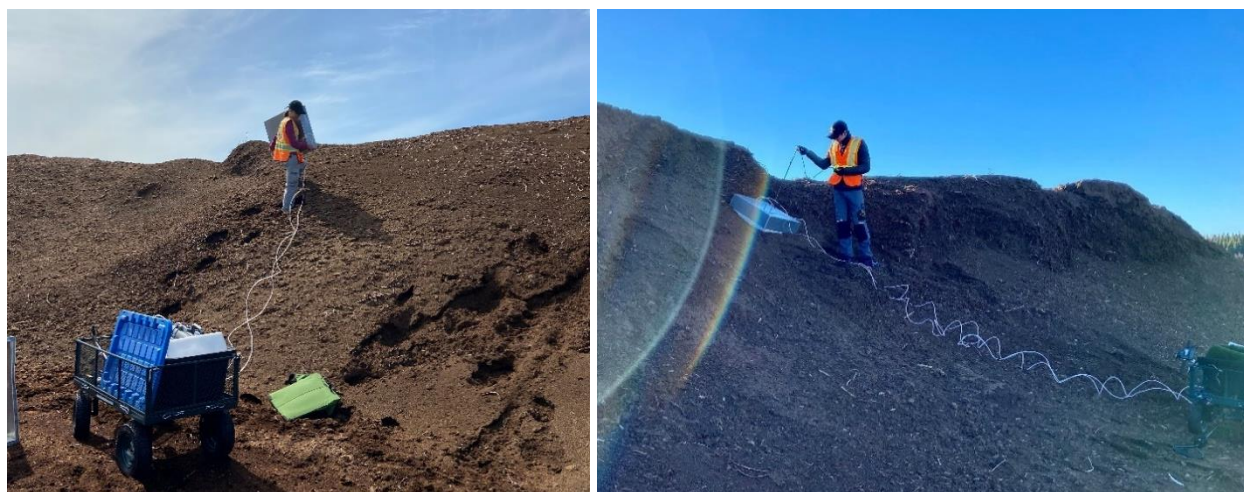
Figure 3.8: Uncovered stockpile flux measurements. Left: holding up the chamber to obtain ambient GHG concentrations, and right: taking temperature measurements next to chamber during a 4-minute flux measurement.
