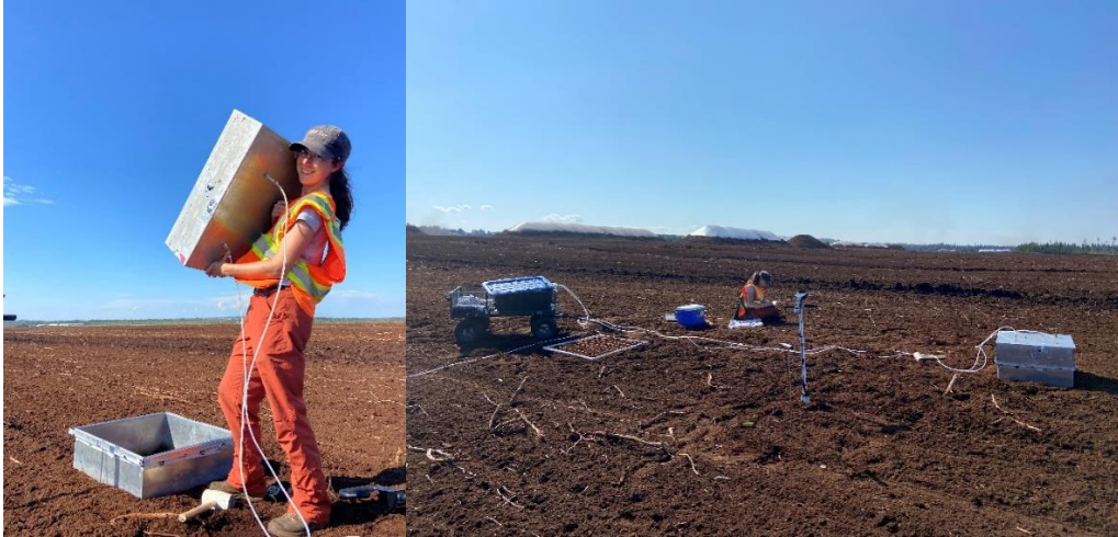
Figure 3.6b: Left: field assistant (C. Jones) holding up the chamber in preparation for a flux measurement. Right: example of flux measurement field setup.
