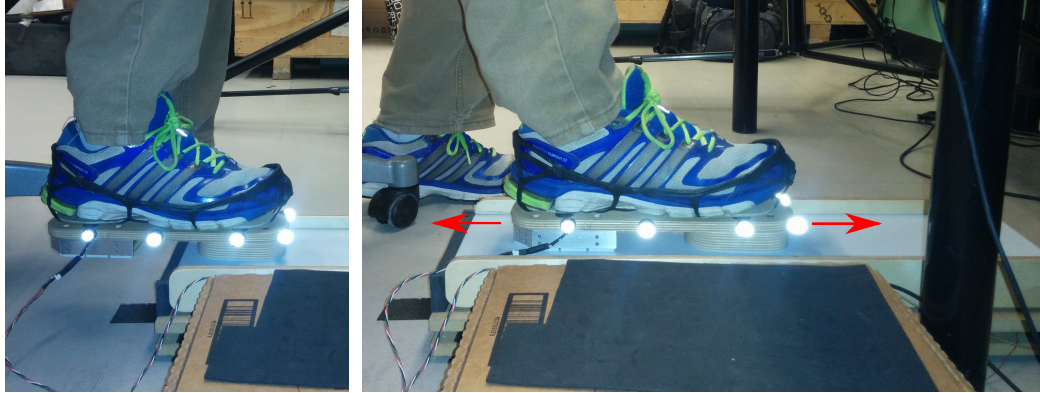
Fig. 4.4: Stimulus selection and testing positions of the foot. As seen in the left image the brake pads were unencumbered during actuation. The image on the right illustrates the motion profile used to test a stimulus.
