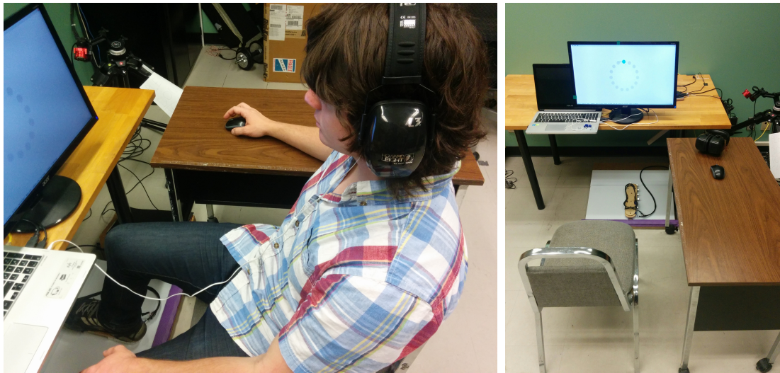
Fig. 5.1: Apparatus used in the foot-controlled pointing Fitts' characterization. The PTFE surface was set on an incline to facilitate a greater range of motion when sliding the foot whilst sitting.
