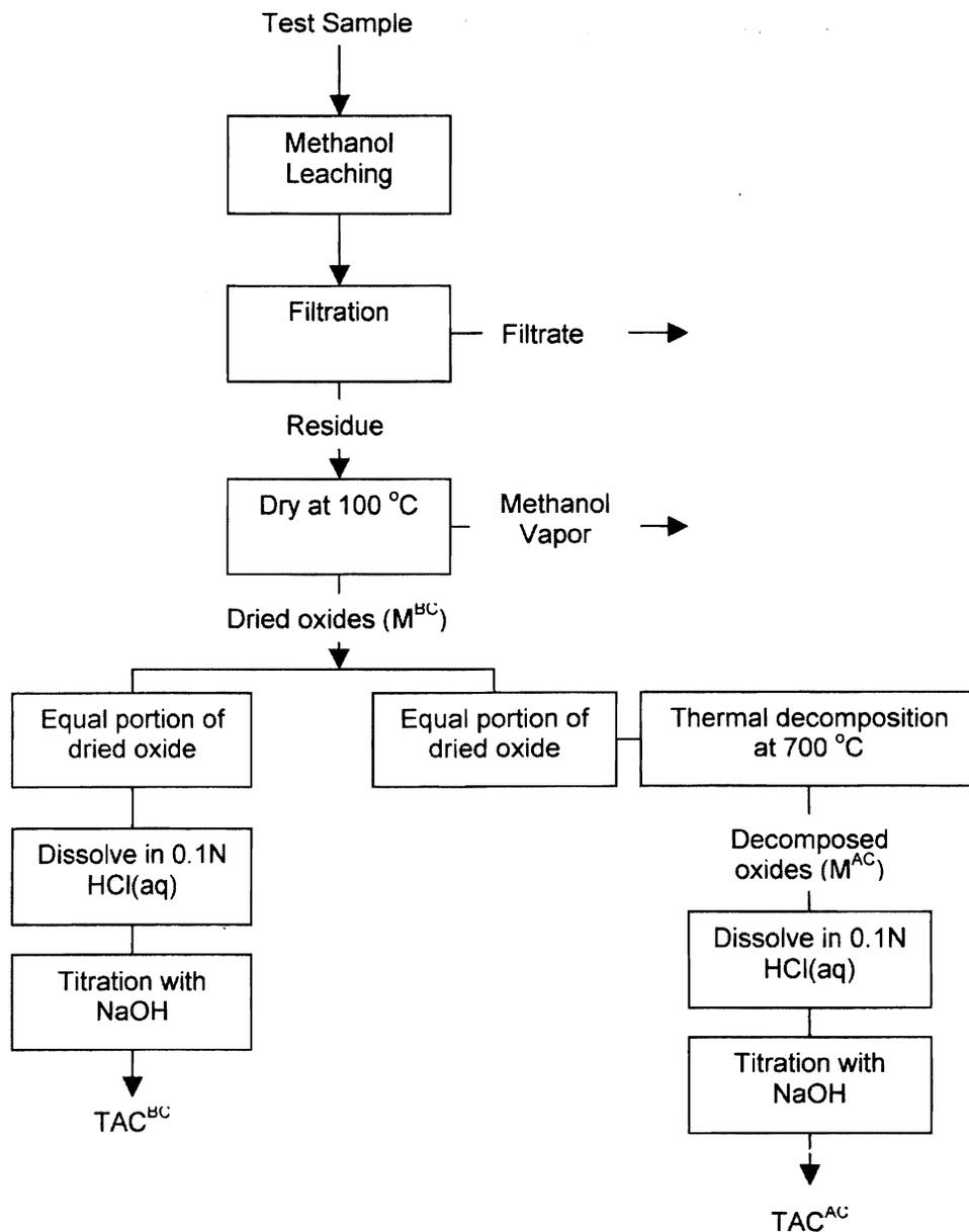
Figure 22: Schematic Representation of the Procedures of the McGill Speciation Technique.
