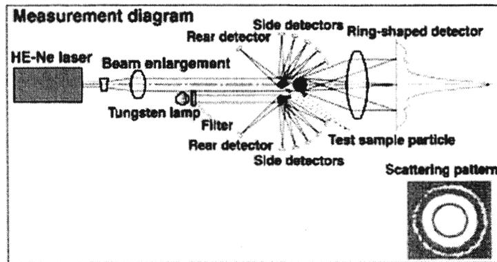
Figure 29: Principal of Laser Particle Size Analysis (LPSA).
