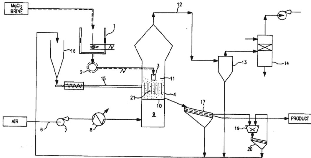
Figure 3: Norsk Hydro Fluidized Bed Prilling Flow Diagram.
