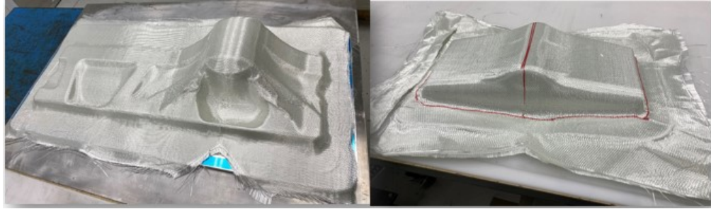
Figure 5-7: Stabilized preform of the horizontal structure (Left) and stabilized preform of the foot structure joined horizontally (Right).
