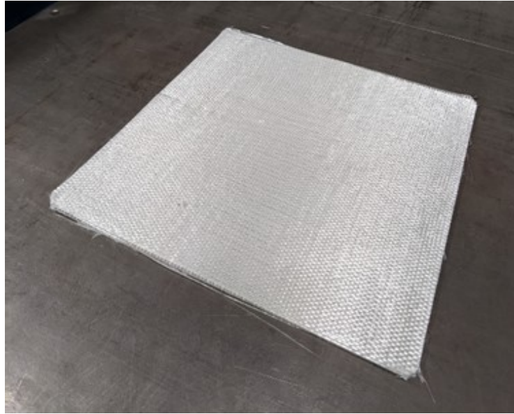
Figure 4-5: TG15N glass NCF after the activation of binder.
