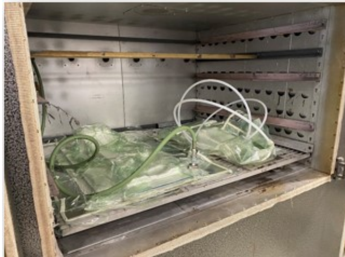
Figure 5-6: Vacuum bagged preform pieces in an oven at 100 °C for binder stabilization.
