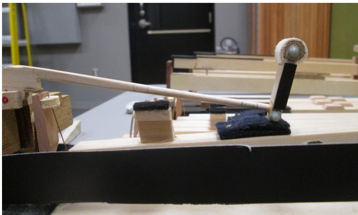
Image 4 – stoss Mechanism with only f2 Hammer
