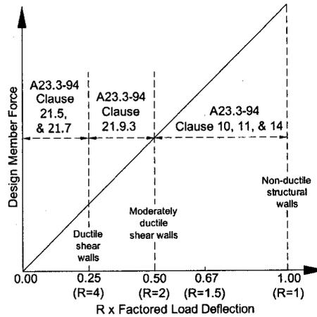
Figure 4-11: Design of reinforced concrete shear walls at various ductility levels (R) according to the CSA A23.3-94 (1994).
