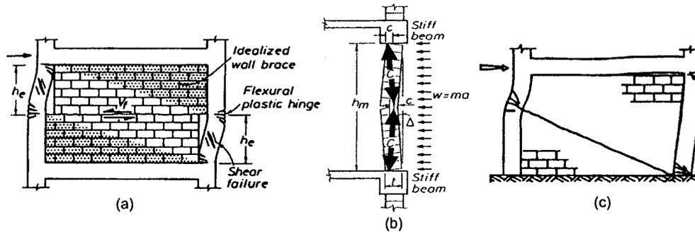
**Figure 1-11: Masonry-infilled frame investigations discussed by various researchers: (a) Sliding shear failure mode and; (b) compression membrane resistance discussed by Paulay and Priestley (1992); (c) diagonal tensile crack failure investigated by Tomažević (1999).**
