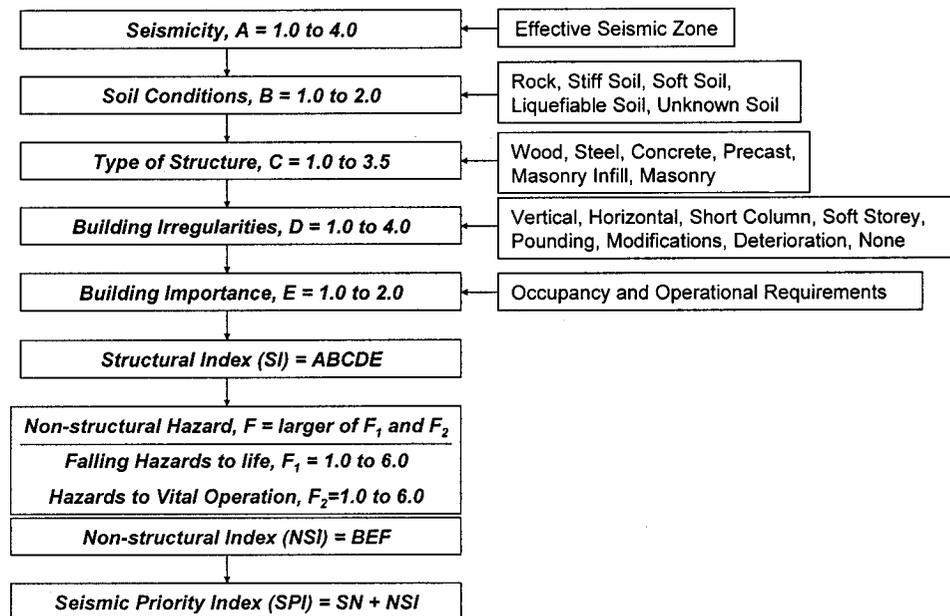
Figure A1: Determination of the NRC SPI index (Foo *et al.*, 2001).
