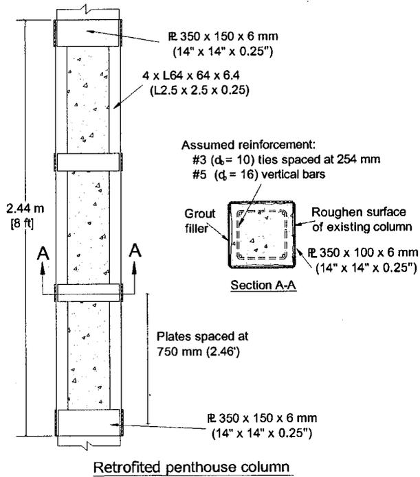
Figure 4-19: Details of penthouse column retrofit.
