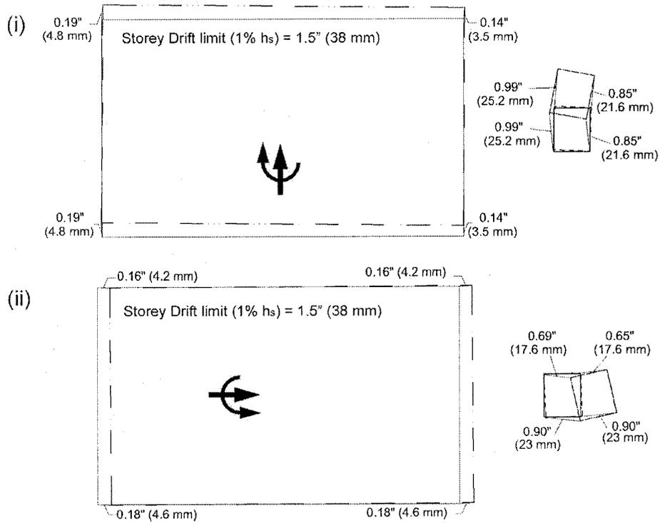
Figure 4-21: The inelastic storey drifts of the retrofitted structure under the full 1995 NBCC design earthquake loads: (i) in the y-direction; and (ii) in the x-direction.
