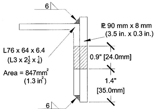
Figure B8: Steel angle reinforced with steel plate at the bolted connection.
