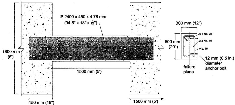
Figure 4-5: A method of repairing coupling beam using bolted steel plates investigated by Mitchell et al., (1996).
