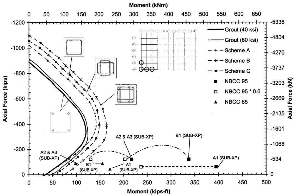
Figure 3-11: Selected analysis results of sub-structure 1 plotted with the nominal sectional resistances of various assumed exterior column sections.
