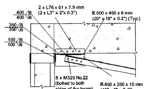
Brace BR1 connection at roof level
