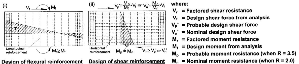
Figure 4-12: Design concept of moment and shear resistances of shear walls.
