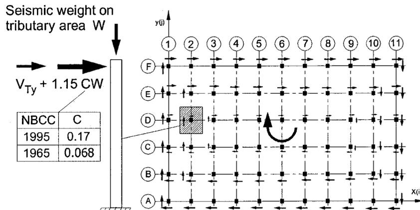
Figure 3-5: The simplified analysis and the additional torsion-induced shear accounted for in the analysis.
