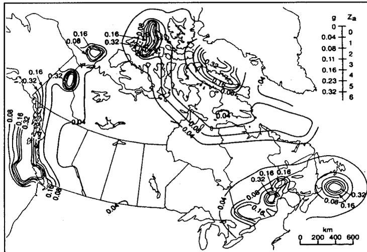
(b-ii) Peak ground acceleration (PGA) contours in 1995 NBCC
