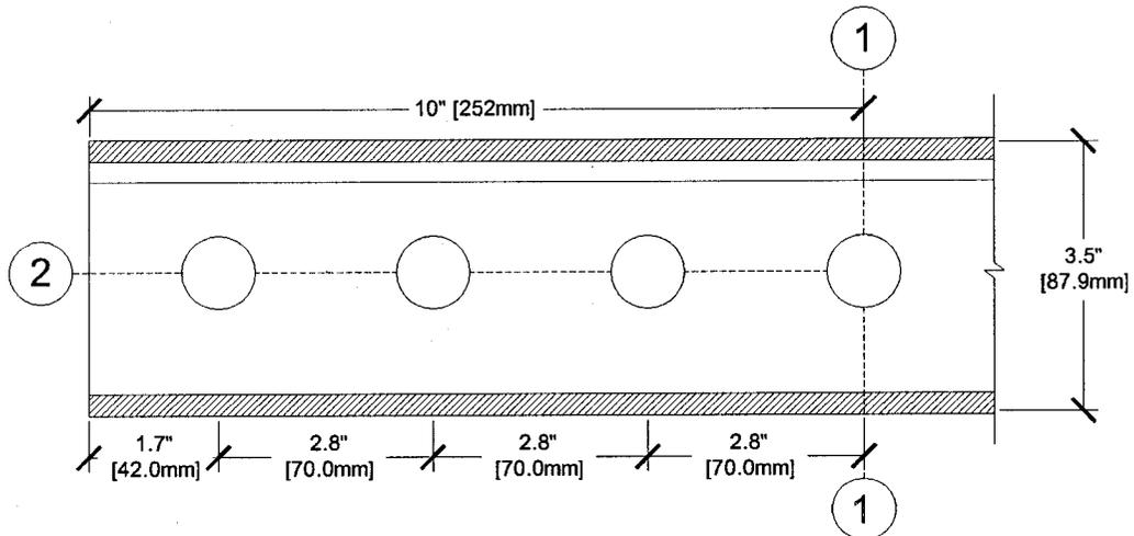
Figure B9: Net section fracture failure paths in the reinforced angle.
