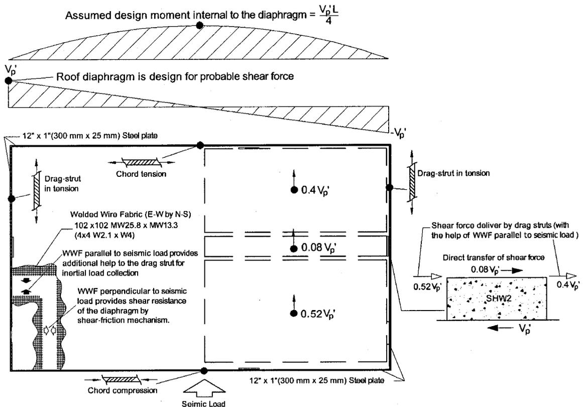
Figure 4-16: Design of the roof diaphragm upgrade.
