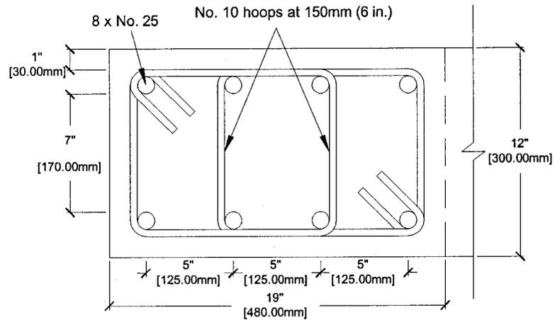
**Figure B1: Details of concentrated reinforcement in the shear walls.**
