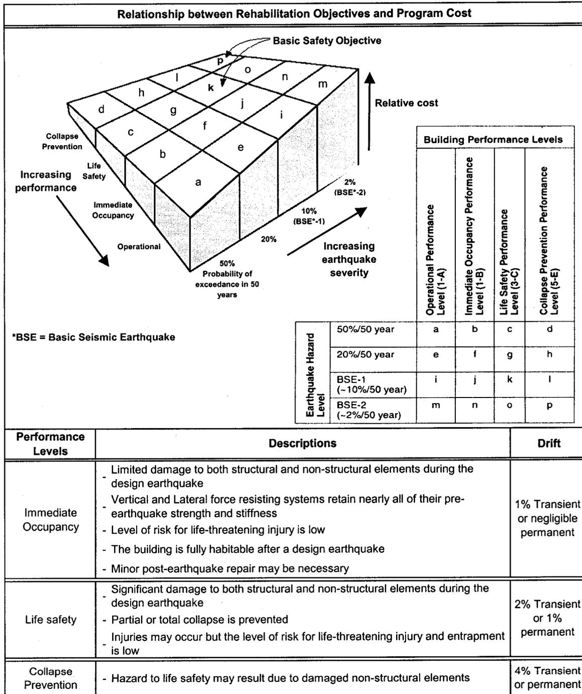
**Figure 1-10: A surface matrix showing the relationships between costs, rehabilitation objectives, seismic hazard levels, and the performance levels emphasized in FEMA 356 (FEMA, 2000).**
