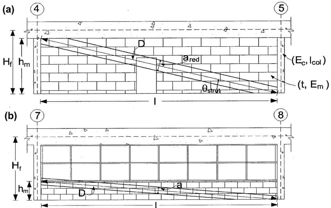
Figure 3-2: Modeling of the masonry-infilled walls: (a) an infilled frame with an opening; (b) a partially infilled frame.
