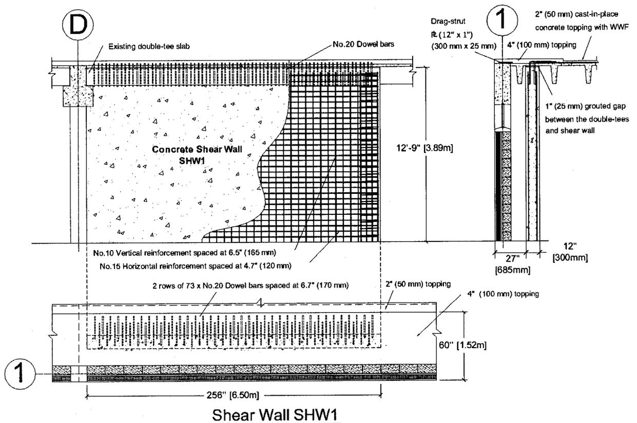
Figure 4-13: Elevation of shear wall SHW1.
