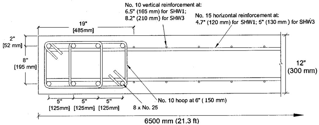
Figure 4-15: Reinforcing details of the shear wall.
