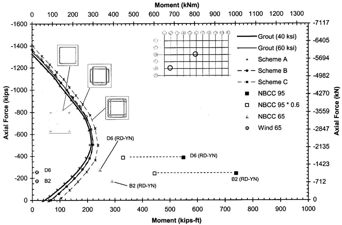
Figure 3-8: Selected rigid diaphragm analysis results plotted with the nominal sectional resistances of various assumed interior column sections.
