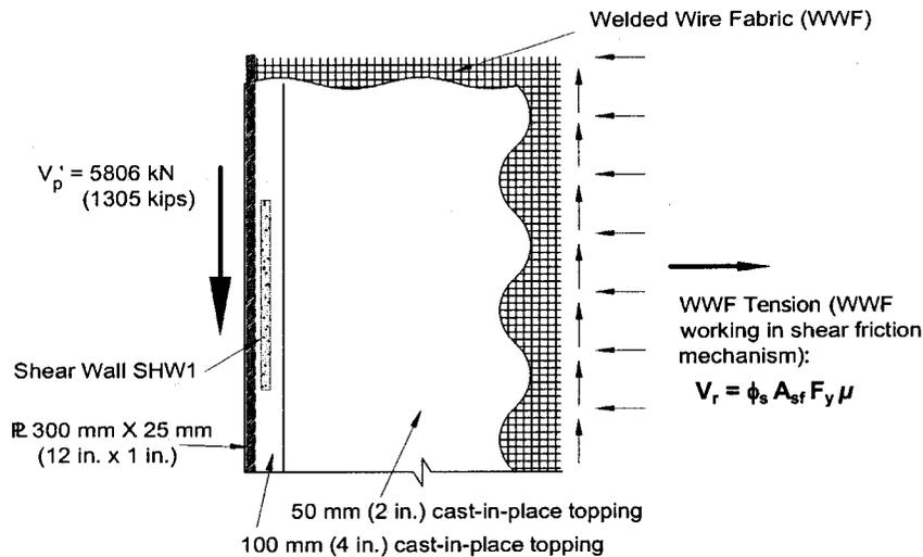
**Figure B2: Shear-friction model for design of topping reinforcement.**
