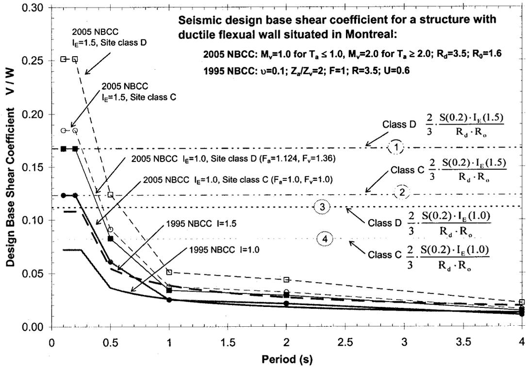
**Figure 4-23: Comparisons of base shear coefficients computed according to the proposed 2005 NBCC and the current 1995 NBCC for a normal and a post-disaster structure located in Montréal.**
