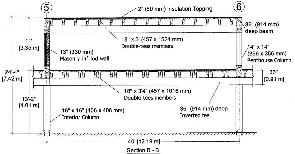
Figure 2-4: Elevation view of Section B-B.
