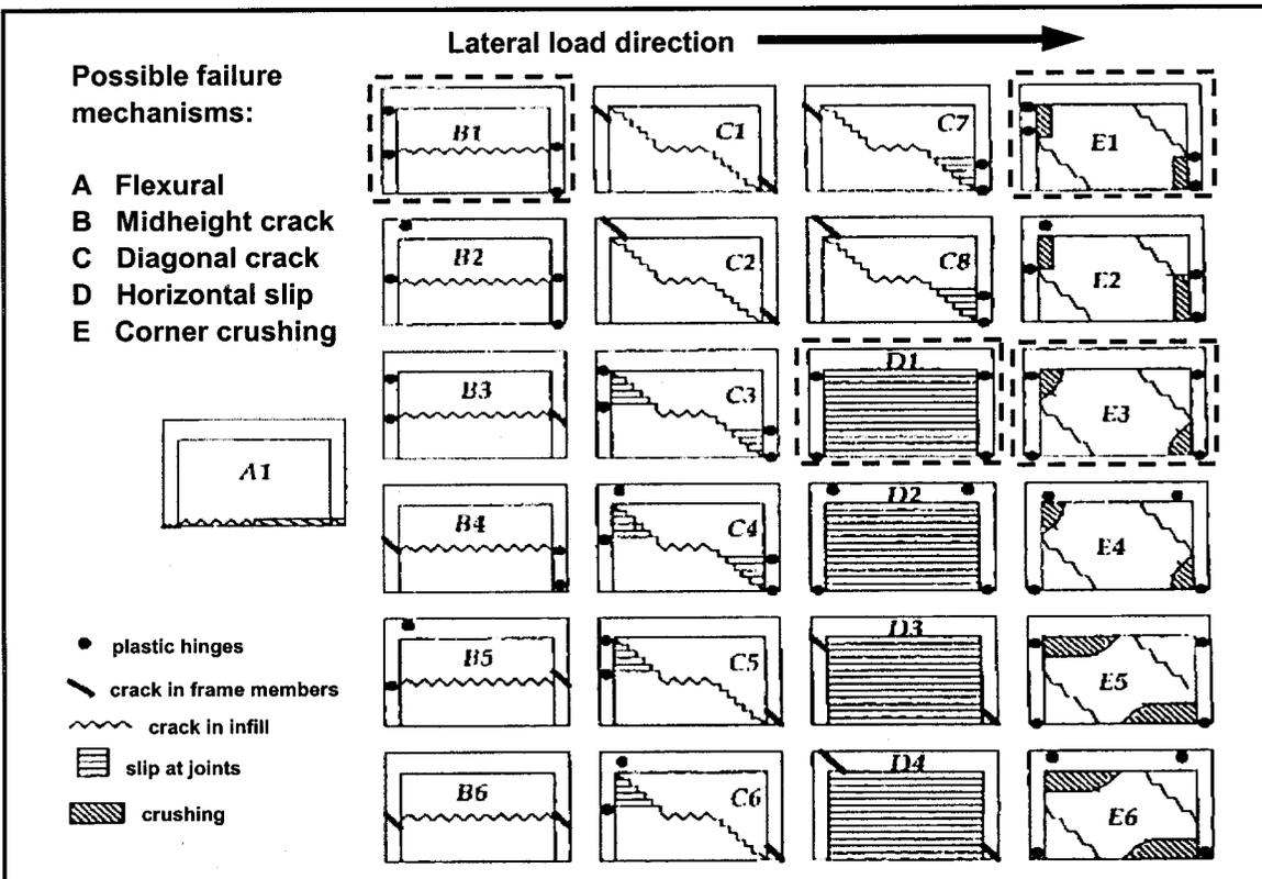
**Table 1-2: Failure modes of masonry-infilled frames summarized from Mehrabi and Shing (2002).**
