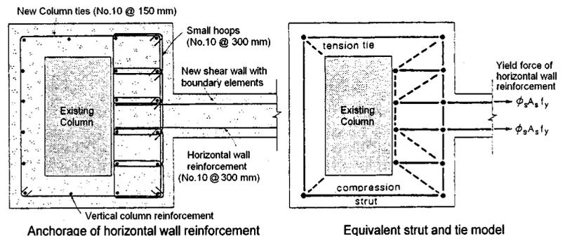
Figure 4-2: Anchorage of horizontal reinforcement for an infilled shear wall with boundary elements (Dandurand, 1988).
