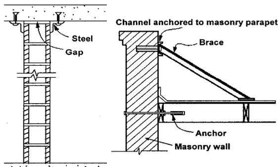
Figure 4-8: Anchorage of masonry wall (Allen, 1993).
