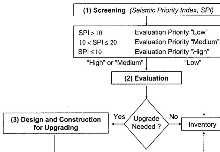
Figure 1-9: The NRC seismic screening procedure (*Foo et al., 2001*).
