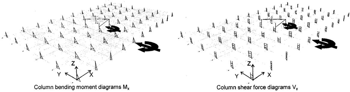
Figure 3-6: Bending moment and shear force distribution in a rigid diaphragm model.
