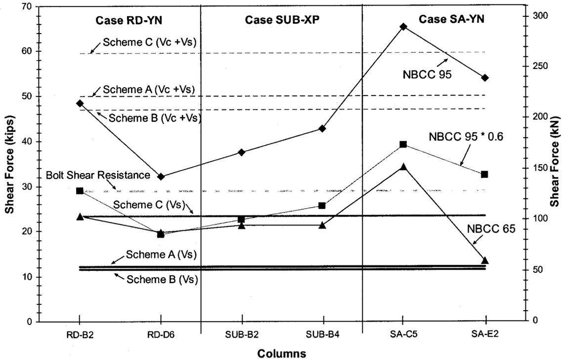
Figure 3-15: Comparison between shear forces and nominal shear resistances of selected interior columns.
