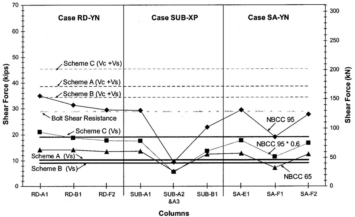
Figure 3-16: Comparison between shear forces and nominal shear resistances of selected exterior columns.
