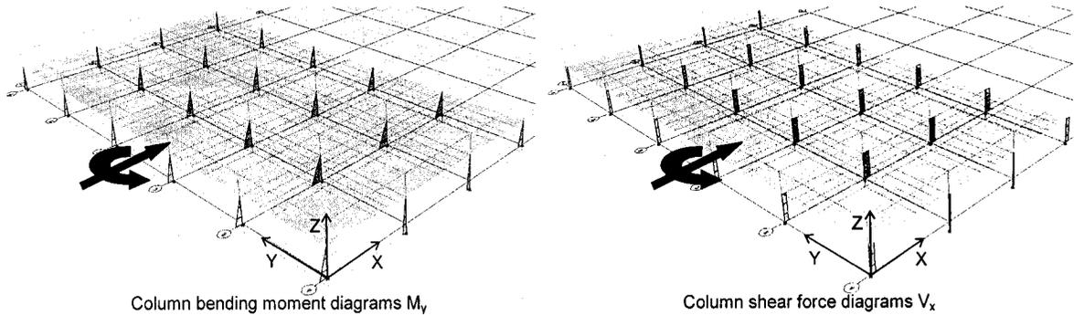
Figure 3-7: Bending moment and shear force distribution in sub-structure 1 model.
