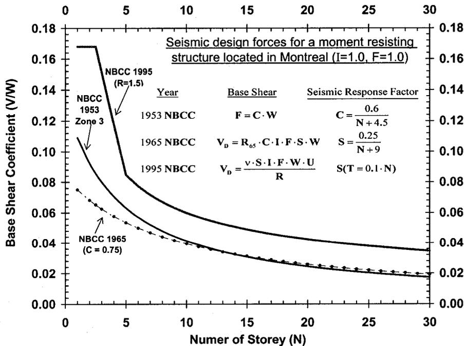
Figure 1-8: Level of seismic design base shear from various editions of NBCC.
