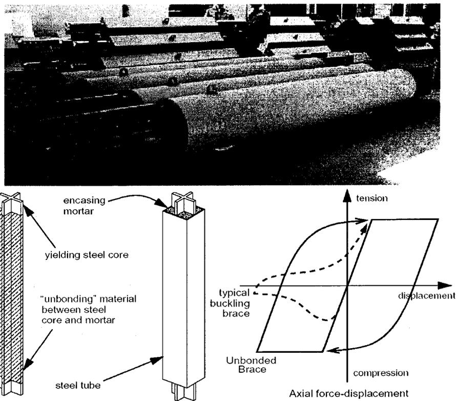
Figure 4-7: Buckling restrained braces (Brown et al., 2001).
