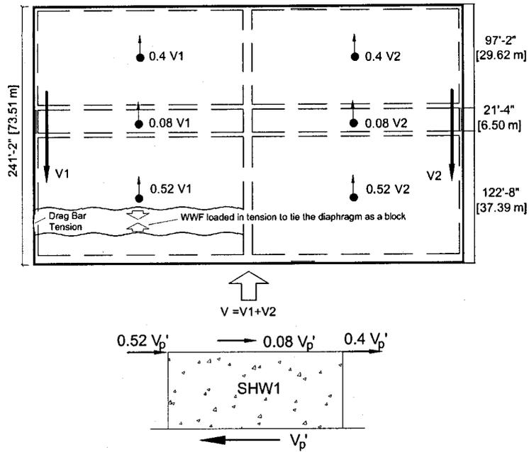
Figure B4: Distribution of earthquake inertial force in the N-S direction.
