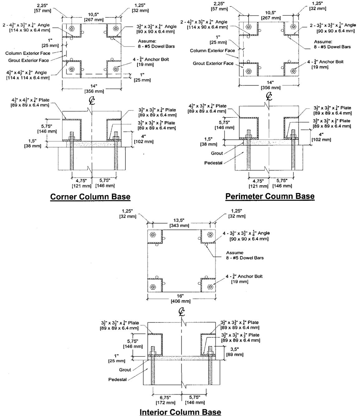
Figure 2-5: Column base connections.
