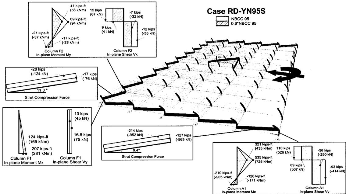
**Figure 3-18: Selected internal force diagrams of members affected by the partially infilled walls in a rigid diaphragm model subjected to y-direction earthquake forces.**
