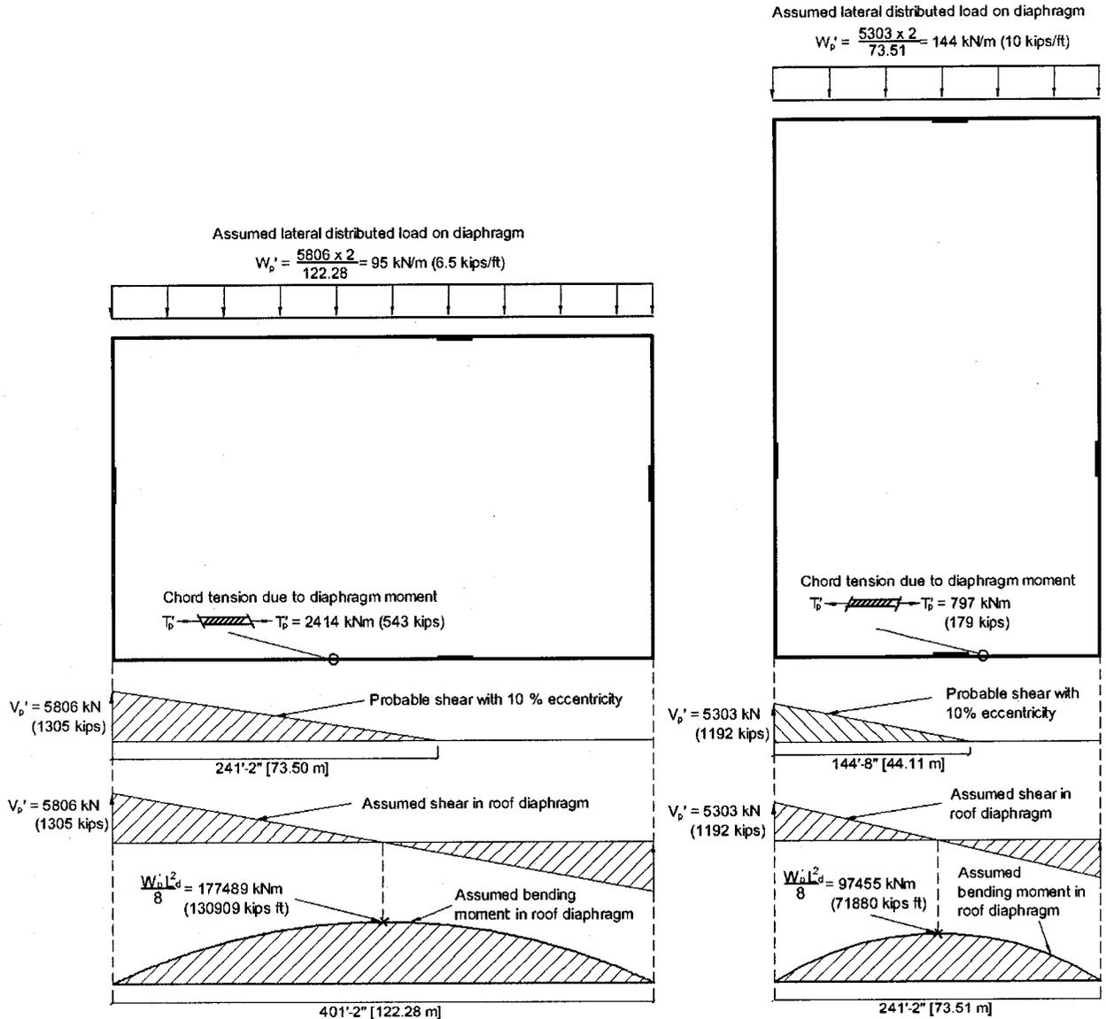
Figure B6: Assumed values of design moments to ensure the elastic behavior of the diaphragm.
