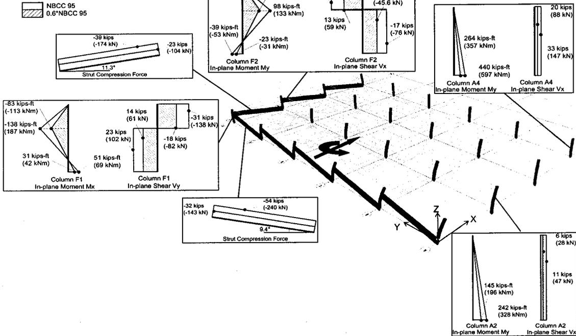
**Figure 3-19: Selected internal force diagrams of members affected by the partially infilled walls in a sub-structure 1 model subjected to x-direction earthquake forces.**
