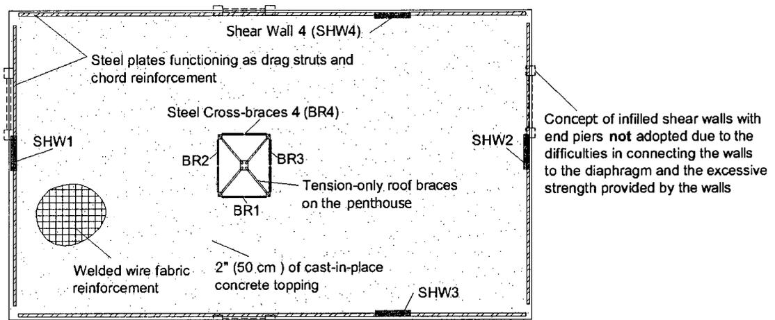
Figure 4-10: Conceptual strengthening scheme for the single-storey warehouse.
