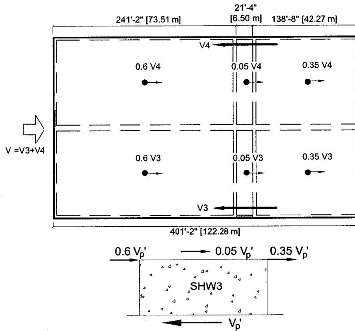
Figure B5: Distribution of earthquake inertial force in the E-W direction.
