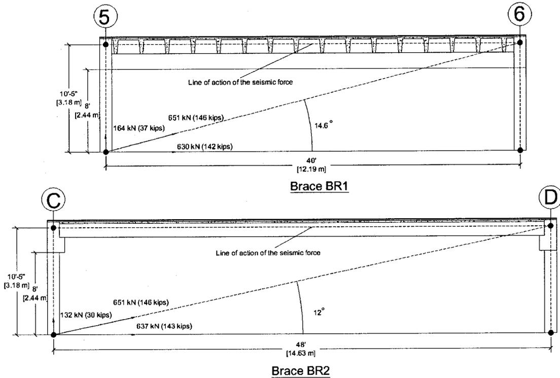
Figure B7: Geometry of the brace bents and probable tensile forces to be resisted by the connections.
