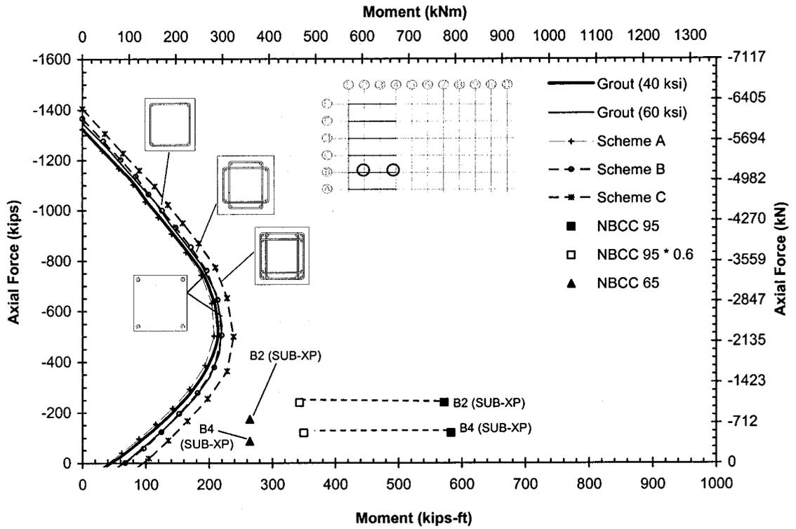
Figure 3-10: Selected analysis results of sub-structure 1 plotted with the nominal sectional resistances of various assumed interior column sections.
