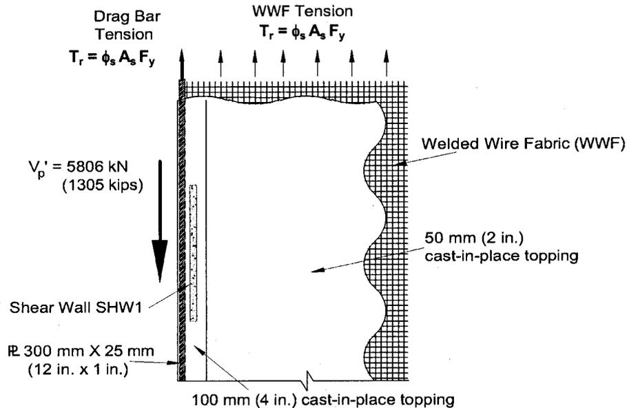
Figure B3: Welded wire fabric assisting the drag bar to transfer diaphragm inertial load.
