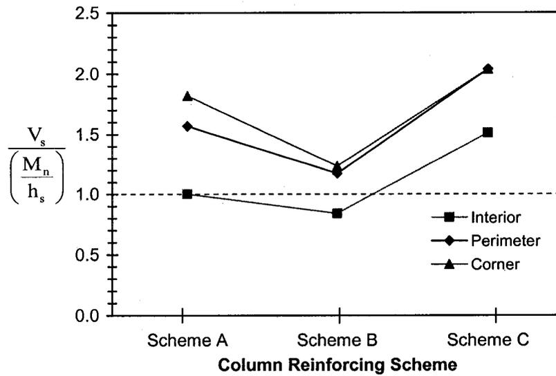
Figure 3-14: Ratio of nominal shear resistances to the shear forces associated with the development of nominal moment resistances for various reinforced column sections.
