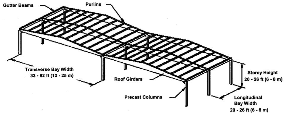
Figure 1-2: Typical single-storey precast concrete structures in Turkey (*Posada & Wood, 2002*).
