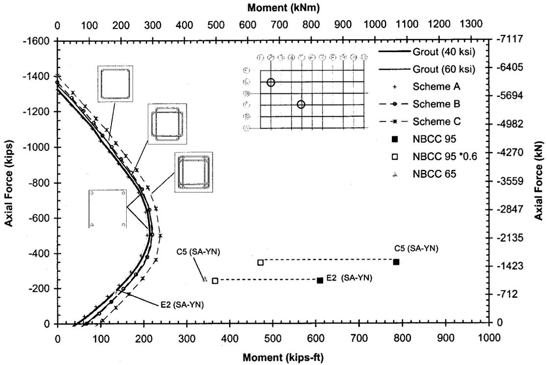
Figure 3-12: Selected results of simplified analysis plotted with the nominal sectional resistances of various assumed interior column sections.
