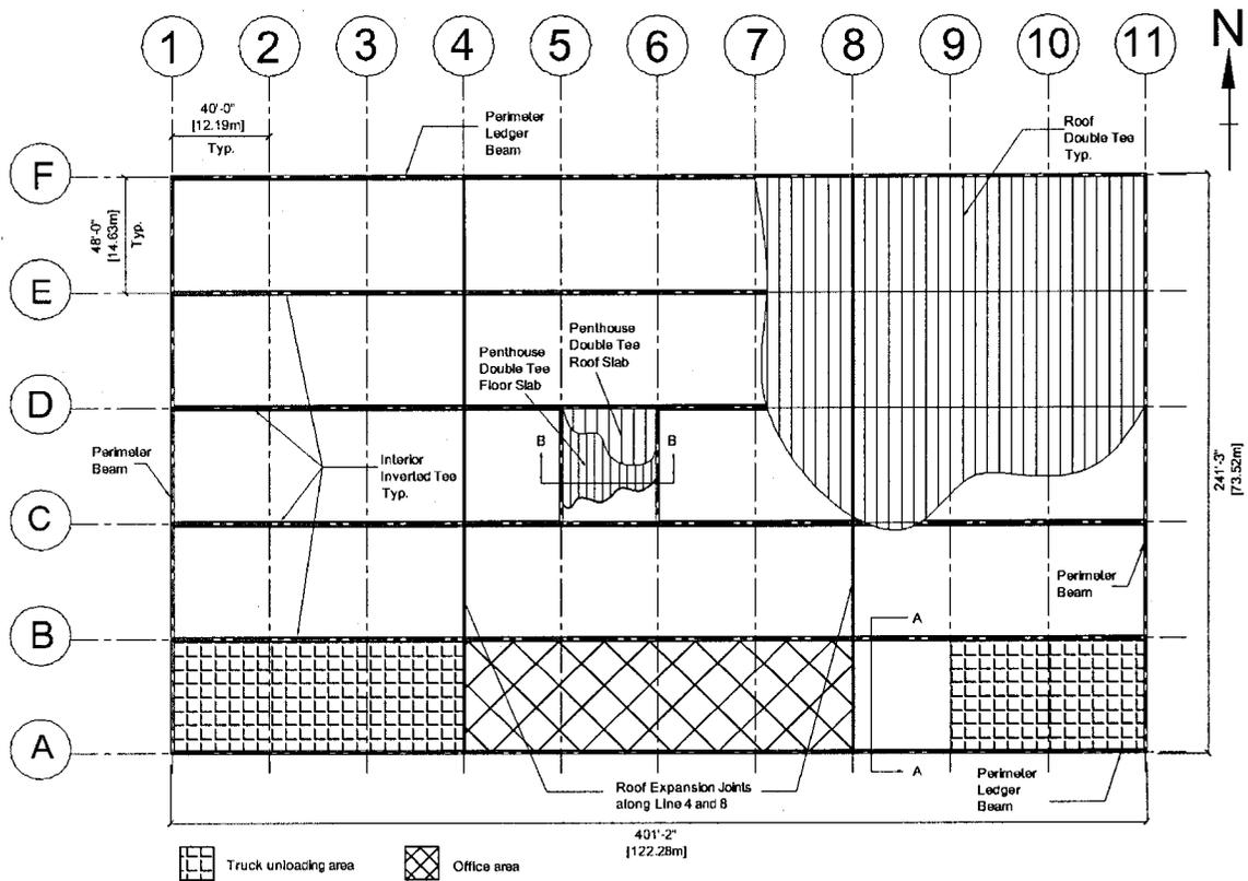
Figure 2-1: Plan view of the warehouse.
