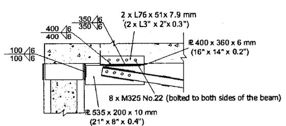
Brace BR2 connection at roof level
