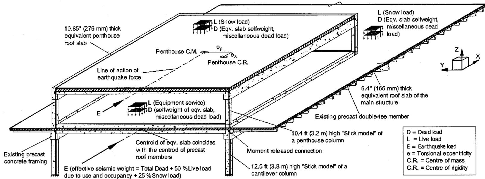
Figure 3-1: Applications of design loads and modeling of the precast framing (masonry-infilled walls not shown).
