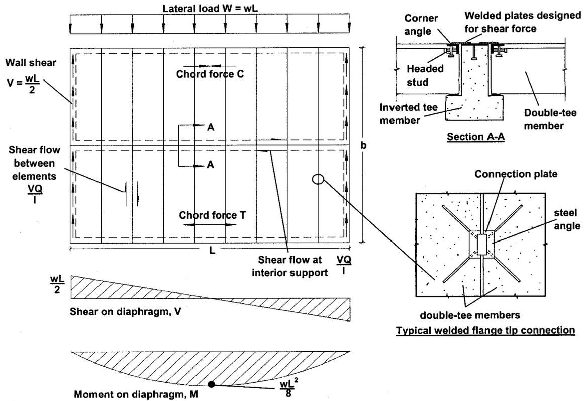
Figure 1-1: Design of precast concrete roof diaphragm (CPCI, 1996).
