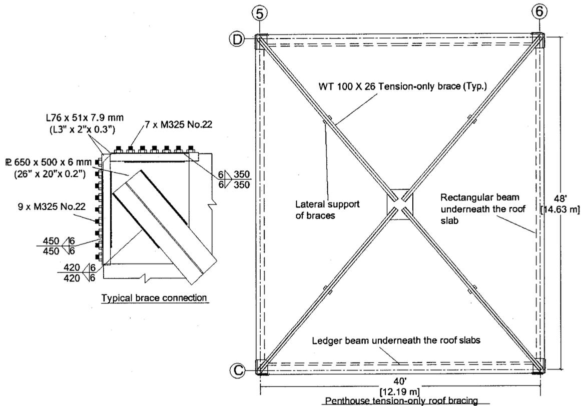
Figure 4-20: Tension-only roof braces on the penthouse.
