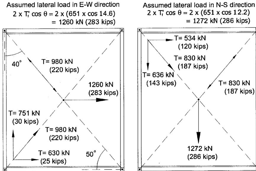
**Figure B10: Assumed design forces acting in the tension-only roof braces.**
