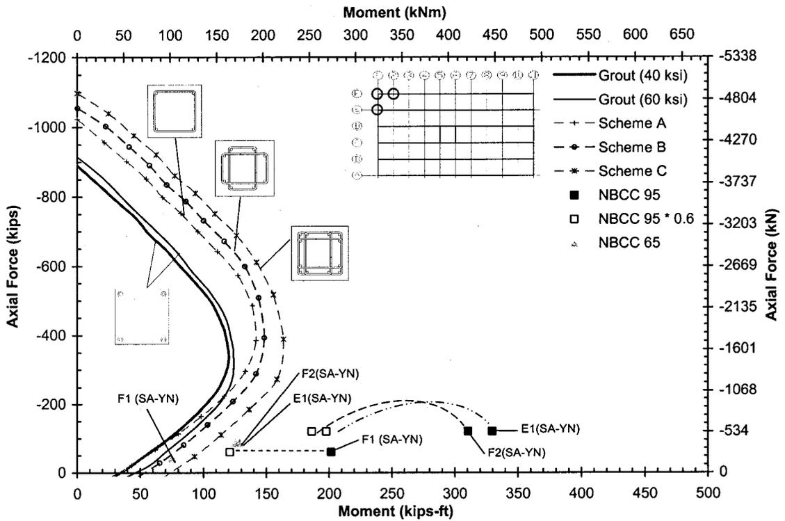
Figure 3-13: Selected results of simplified analysis plotted with the nominal sectional resistances of various assumed exterior column sections.
