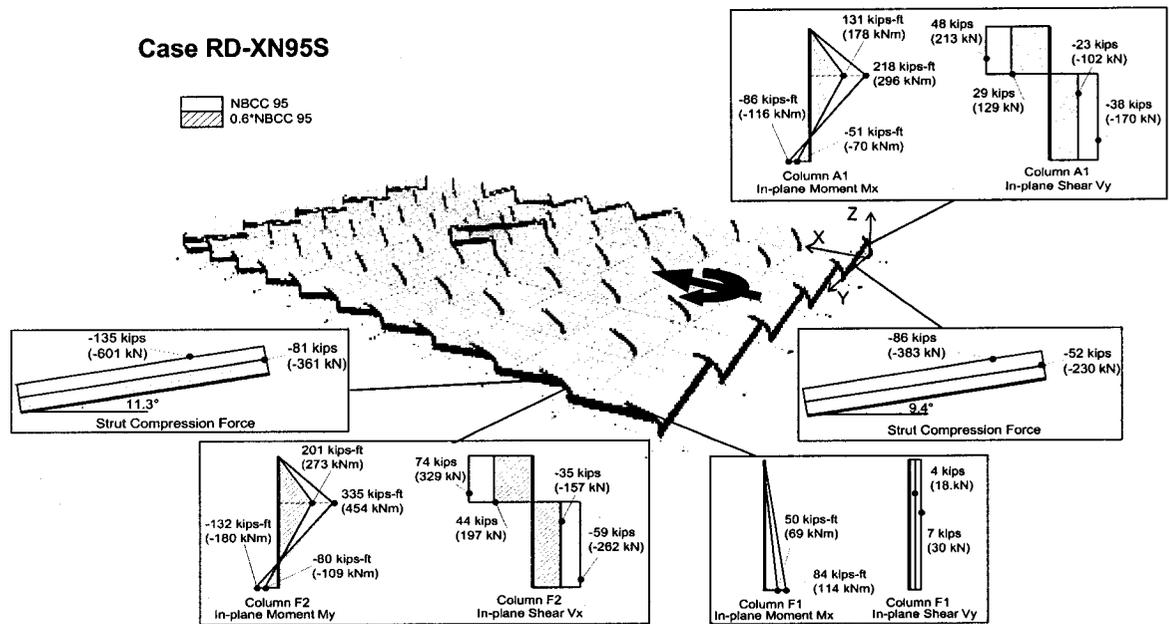
**Figure 3-17: Selected internal force diagrams of members affected by the partially infilled walls in a rigid diaphragm model subjected to x-direction earthquake forces.**
