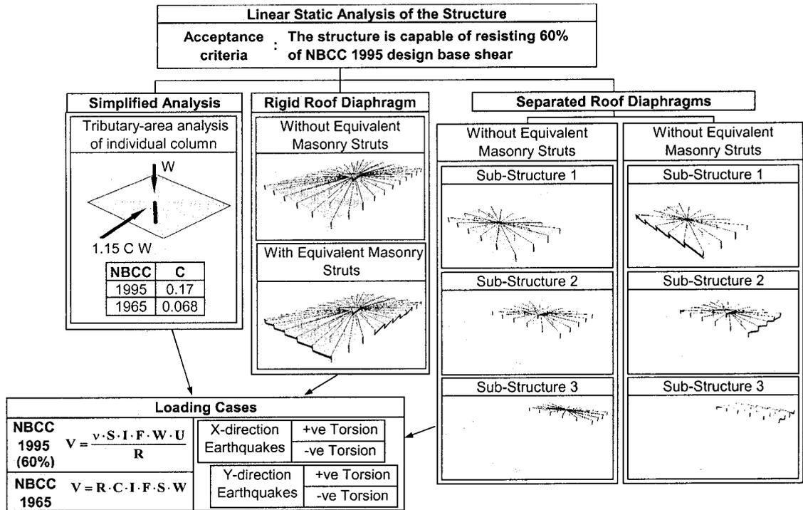
Figure 3-3: Analysis methodology used in seismic evaluation of the warehouse.
