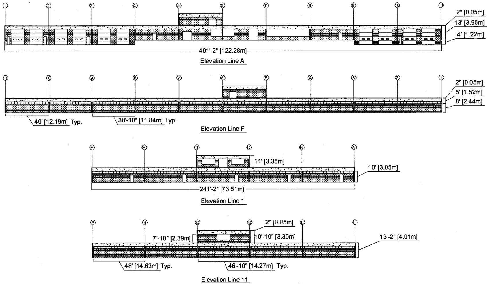
Figure 2-2: Elevation views of the warehouse.
