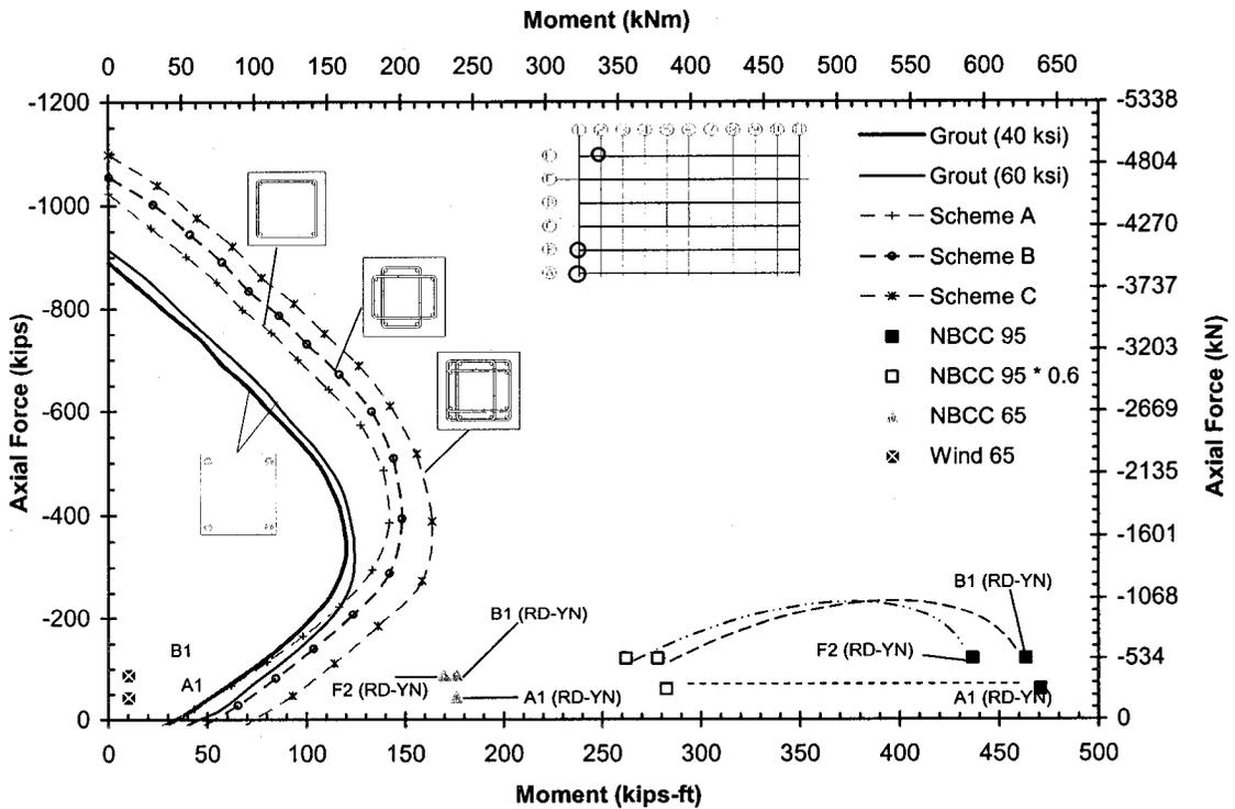
Figure 3-9: Selected rigid diaphragm analysis results plotted with the nominal sectional resistances of various assumed exterior column sections.
