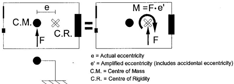
Figure 3-4: Schematic diagram showing the application of earthquake forces on a single-storey structure with a rigid diaphragm.
