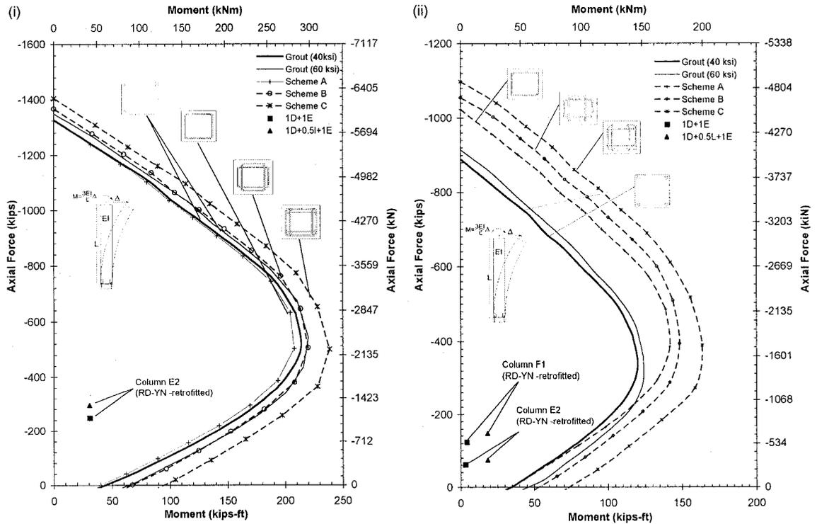
Figure 4-22: Deflection induced moment and gravity load in selected (i) interior columns; and (ii) exterior columns (values of the column deflections correspond to those recorded in Figure 4-21 (i)).
