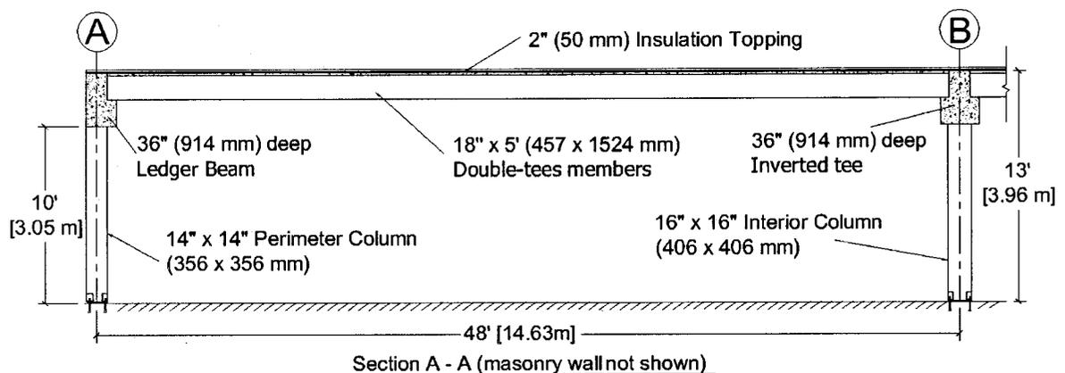
Figure 2-3: Elevation view of Section A-A.
