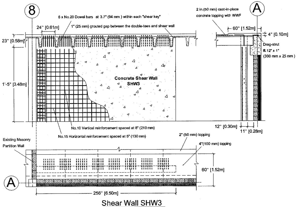
Figure 4-14: Elevation of shear wall SHW3.
