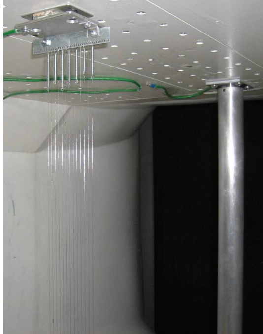
Figure 2.3: The mandoline (top half seen on the left) placed in front of the cylinder
