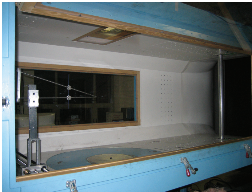
Figure 2.2: The cylinder (seen on the right) placed in the test section of the wind tunnel
