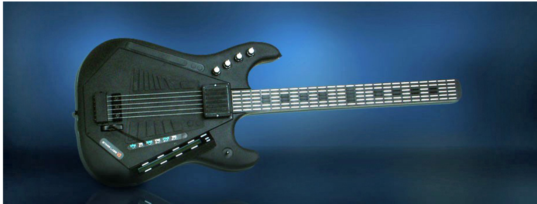
(c) A Ztar Mark III V3 MIDI guitar controller designed by Starr Labs.
