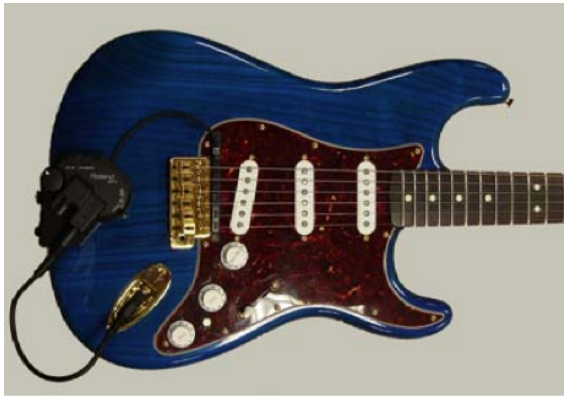
(a) Hexaphonic pickup (Roland GK-3) installed on a Fender Deluxe Player Stratocaster (O’Grady and Rickard 2009).
