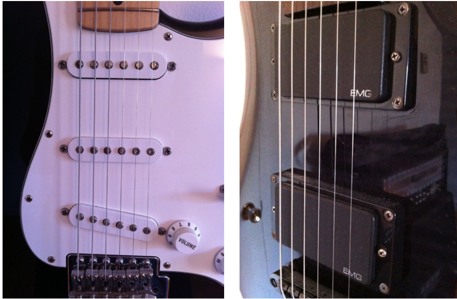
(a) Array of single-coil pickups on a Fender Stratocaster. (b) Array of EMG-81 active dual-coil covered pickups on an LTD F-400FM.
