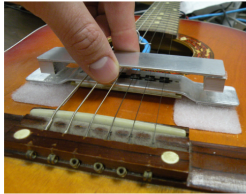
(b) Sensor mount and reflective surface installed on a Cameo acoustic guitar (Fitzgerald et al. 2011).
