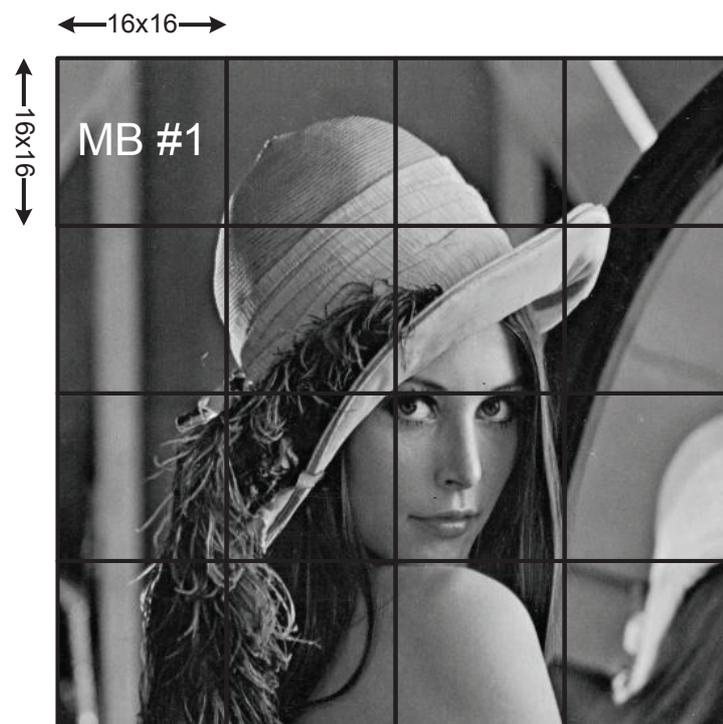
**Figure 2.4** An arbitrary frame divided into macroblocks each of size  $16 \times 16$  pixels.
