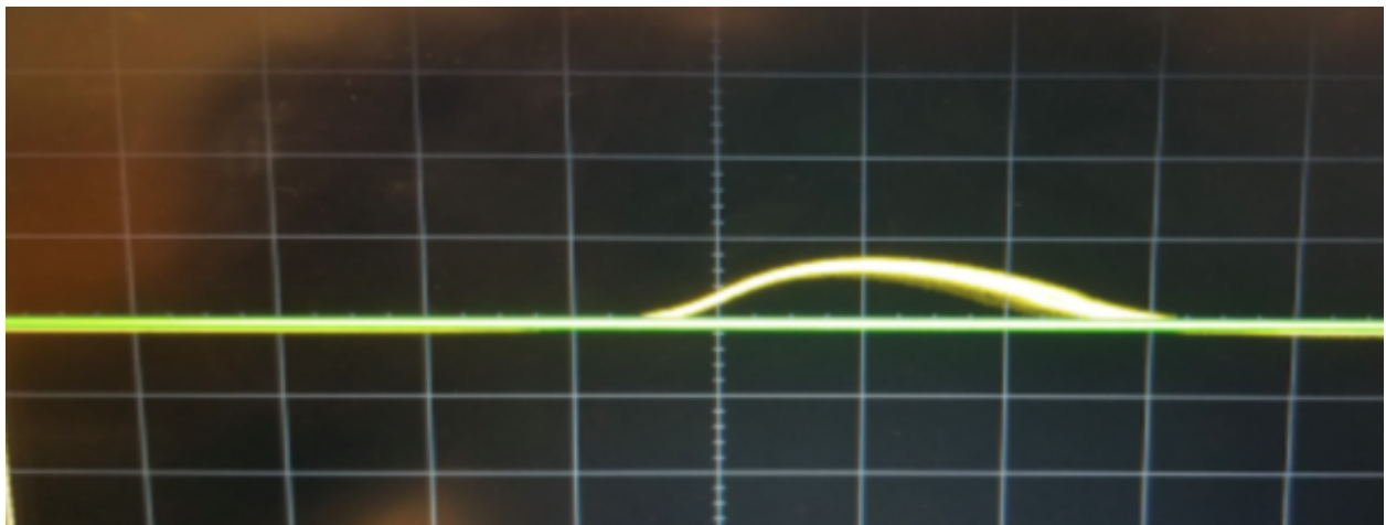
Fig 23: Simulation results for the two amplifier circuits (upper) Output of the two-amplifiers gain stage when the photodetector is saturated with light at 840 ns/div with 1.8 V (lower)
