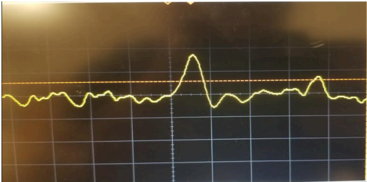
Fig 26: The output of the leading-edge discriminator at 20 ns/div with a 4.8 V
