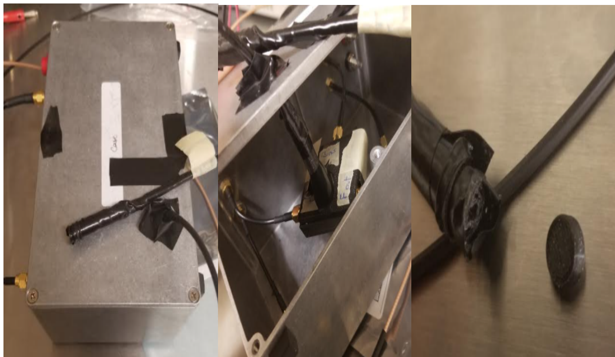
Fig 11: The photodetector is enclosed in the metal box. Light is guided by the optical fiber (right) to the photodetector enclosed in the case (middle)
